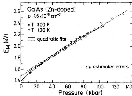
FIG. 6. Pressure dependence of the emission-peak maximum  $E_M$  at low and room temperature for  $p$ -GaAs with  $1.6 \times 10^{19}$  holes  $\text{cm}^{-3}$ . At 120 K the direct gap depends linearly on pressure, while at 300 K a sublinear behavior is observed. The quadratic fits were performed with Eq. (6) and the obtained pressure coefficients are summarized in Table III.
