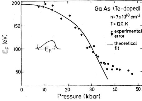
FIG. 10. Pressure dependence of the Fermi level ( $E_F$ ) measured from the bottom of the conduction band  $\Gamma_1^c$  in  $n$ -GaAs with  $7 \times 10^{18}$  electron  $\text{cm}^{-3}$ .  $E_F$  was determined from the difference between the optical gap and the direct gap with Eq. (8). The theoretical fit was performed in a way described in the Appendix.
