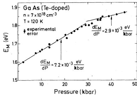
FIG. 11. Pressure dependence of the emission at  $T = 120$  K around the direct gap  $E_0$  in heavily doped  $n$ -GaAs. With increasing pressure the emission shifts to higher energies with a smaller pressure coefficient than that of the  $p$  samples at the same temperature. This behavior is explained considering the pressure dependence of the Fermi level.
