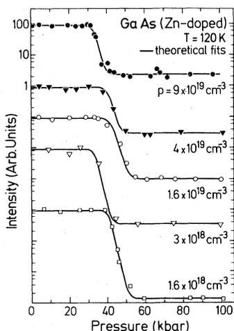
FIG. 2. Pressure dependence of the emission across the  $E_0$  gap for a series of hole concentrations. For each hole concentration the vertical scale has been displaced. The solid lines correspond to fits performed with Eq. (1). The obtained parameters are listed in Table I.
