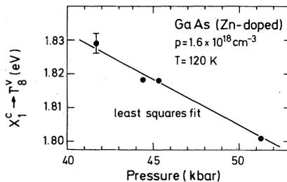
FIG. 5. Pressure dependence of the  $X_1^c \rightarrow \Gamma_8^v$  emission line described in Fig. 4. The solid line represents a least squares fit with Eq. (5).
