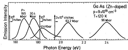
FIG. 1. Typical emission spectra around the  $E_0$  direct gap as a function of pressure at 120 K for a heavily Zn-doped  $p$ -GaAs with  $9 \times 10^{19}$  holes  $\text{cm}^{-3}$ . With increasing pressure the emission lines shift to higher energies. Their intensity decreases for pressures between 30 and 45 kbar because of the " $\Gamma_1^c, X_1^c$ " crossing. Although the material becomes indirect after this crossing, the emission from  $E_0$  can still be observed.
