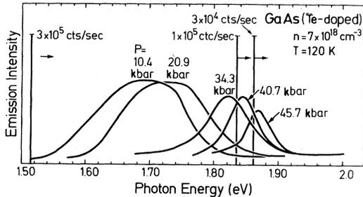
FIG. 8. Typical emission lines at  $T=120$  K across the direct gap  $E_0$  in  $n$ -type GaAs for various pressures. With increasing pressure the intensity of the lines decreases and they become narrower. Both effects can be related to the transfer of the free electrons from the  $\Gamma_1^c$  states to the  $X_1^c$  minima.
