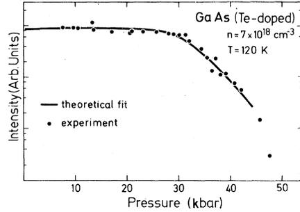
FIG. 9. Pressure dependence of the emission intensity across the direct gap  $E_0$  in  $n$ -type GaAs. The emission cannot be observed after the gap becomes indirect. The solid line is a theoretical fit with Eq. (7).
