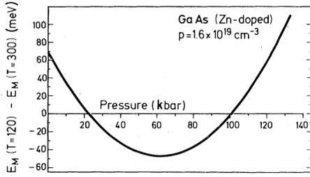
FIG. 7. Energy difference at  $T=120$  and  $300$  K of the emission lines across the direct gap as a function of pressure.
