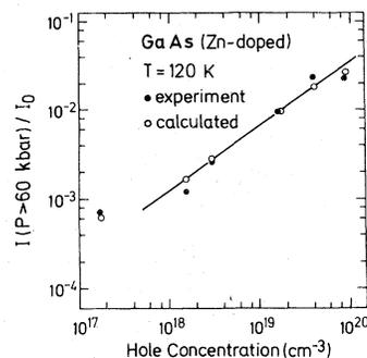
FIG. 3. Hole-concentration dependence of the intensity of the  $E_0$  luminescence for pressures above 60 kbar normalized to that at very low pressures. The calculated points were obtained with Eq. (4). The solid line has been drawn as a visual aid.
