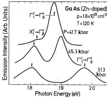
FIG. 4. Typical luminescence spectra at 120 K from the samples with  $1.6 \times 10^{18}$  holes  $\text{cm}^{-3}$  for pressures between 40 and 55 kbar. They show two lines. One corresponds to emission from the direct gap  $E_0$  ( $\Gamma_1^c - \Gamma_8^v$ ); it shifts to higher energies with pressure. The other line shifts to lower energies with increasing pressure and is related to indirect transitions across the  $X_1^c - \Gamma_8^v$  indirect gap.
