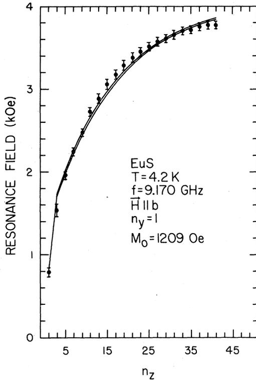
FIG. 3. Comparison of the observed (circles) and calculated (solid lines) resonance fields for various modes  $(1, n_z)$  for  $\vec{H} \parallel b$ . The two solid lines bracket the calculated values, with allowance for the nonuniformity of the sample dimensions.
