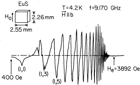
FIG. 2. A copy of the chart recording of the modes, with first few modes labeled. The edge position  $H_e$  and the resonance fields for various modes were determined from separate expanded sweeps.
