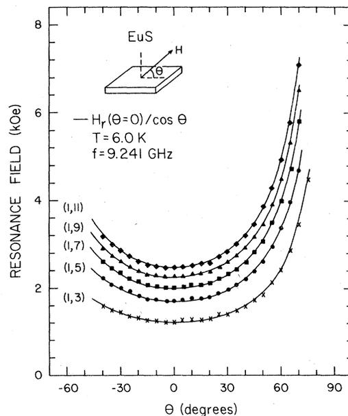
FIG. 7. Angular variation of the resonance field  $H_r$  for several modes as the magnetic field is rotated out of the plane of the platelet.
