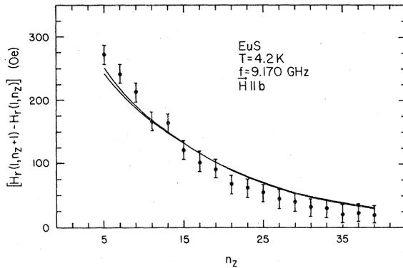
FIG. 5. Magnetic field separation between the consecutive modes vs mode number for  $\vec{H} \parallel b$ . The two solid lines bracket the theoretical predictions.
