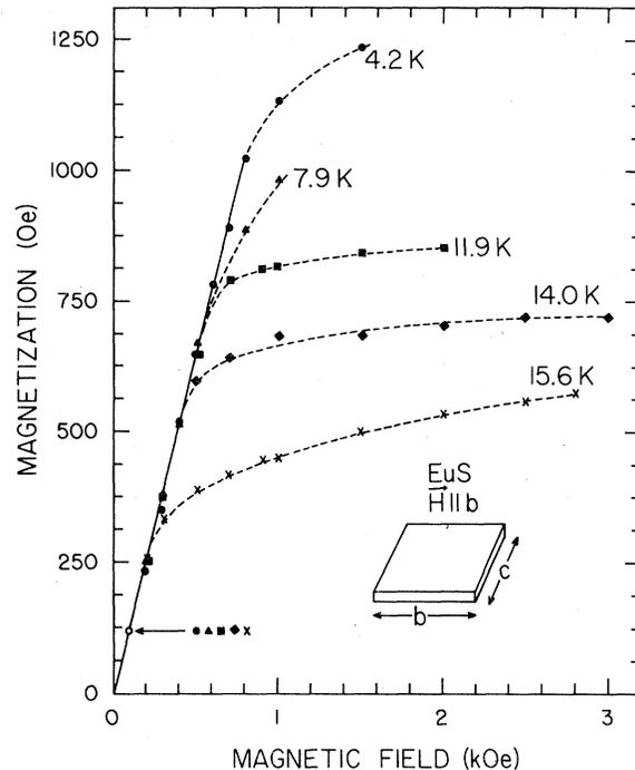
FIG. 1. Magnetization vs applied field at several temperatures for  $\vec{H} \parallel b$ . The dimensions of the nearly square platelet are:  $b = 2.26$  mm,  $c = 2.55-2.65$  mm, and thickness =  $189-196 \mu\text{m}$ . A density of 5.748 for EuS is used to determine the thickness and to obtain the magnetization from the measured (per gram) values. The solid line gives the initial susceptibility and the dotted lines are drawn through the points for visual aid.
