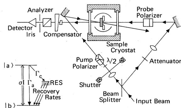
FIG. 1. Apparatus for reading and writing anisotropic holes in a zero-phonon absorption line. The pump beam is polarized in the plane of the page, while the analyzer transmits light polarized perpendicular to that plane. The pump beam is polarized at 45° to the probe. The inset shows the energy-level diagram used to model the hole-writing process. The rates at which the population reservoirs empty into the ground state are much slower than all of the other rates.
