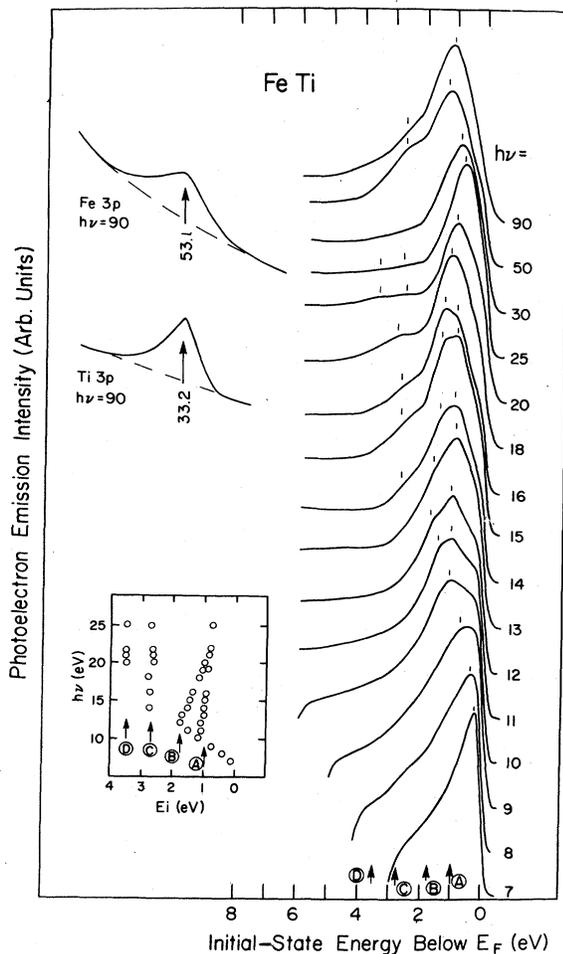
FIG. 1. Photoelectron energy distributions for FeTi for photon energies between 7 and 90 eV. The structure plot in the inset shows the  $h\nu$  behavior of maxima in the PED's. Four features can be identified (arrows) at -1 eV (A), -1.7 eV (B), -2.7 eV (C), and -3.5 eV (D). Core-level features for the Ti and Fe 3p's are shown for  $h\nu=90$  eV with the same energy increments as for the conduction band.
