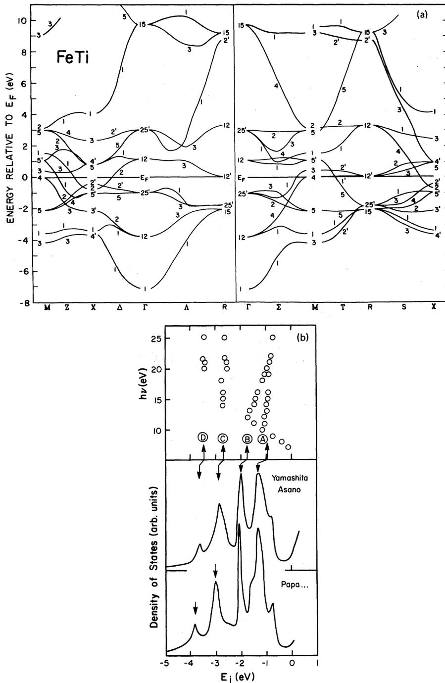
FIG. 2. (a) Calculated band structures of FeTi by Papaconstantopoulos (Ref. 3). (b) The density of states calculated from the bands of (a) (Papaconstantopoulos) compared to that calculated by Yamashita and Asano (Ref. 2) and our experimental results.
