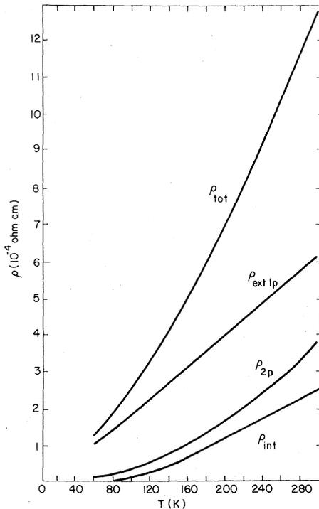
FIG. 6. Calculated  $\rho_v$  versus temperature with  $1p$  and  $2p$  scattering (case II), the latter chosen arbitrarily to contribute  $\sim \frac{1}{3}$  of  $\rho_v$ , for the parameters of Tables I and II. The lower curves give the breakdown into the different scattering processes.
