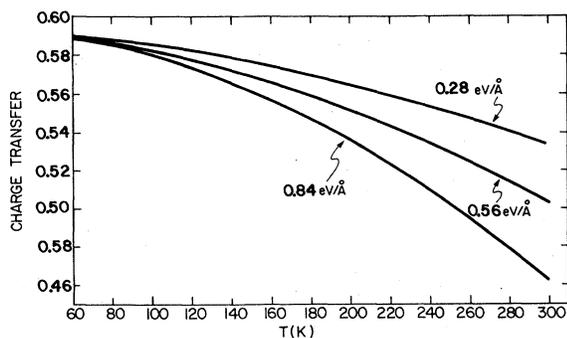
FIG. 3. Calculated variation of charge transfer with temperature for three different values of  $\partial\epsilon_0/\partial b$ .
