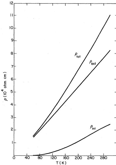
FIG. 4. Calculated resistivity at constant volume  $\rho_v$  including only 1p processes (case I) with the parameters of Tables I and II, and breakdown into external- and internal-mode scattering.
