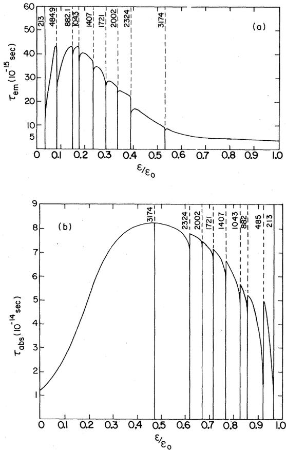
FIG. 2.  $\tau_{em}$  (a) and  $\tau_{abs}$  (b) of Eqs. (2.32) and (2.33), respectively, plotted for  $T = 300$  K,  $\epsilon_0 = 6000$  K,  $\epsilon_F = 1200$  K, and internal-mode frequencies and coupling constants of Table I for TCNQ.
