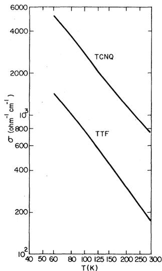
FIG. 5. Separate contributions to  $\sigma$  at constant volume of the TTF and TCNQ chains for the calculation with 1p processes only (case I).
