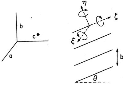
FIG. 1. Coordinate system and model chain of planar molecules showing tilt angle  $\theta$ , lattice constant  $b$ , and rotation axes for the librations.  $\xi$  and  $\zeta$  ( $\parallel a$ ) correspond to the long and short axes of the molecule, respectively, and  $\eta$  to the axis perpendicular to the plane of the molecule.
