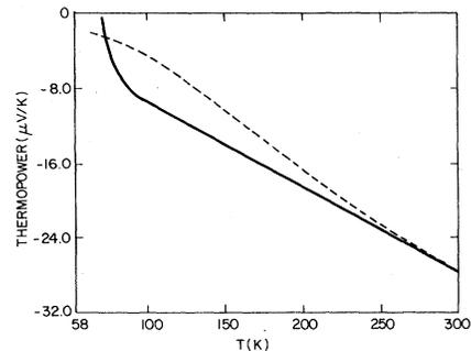
FIG. 8. Measured thermopower (solid line, taken from Ref. 43) and calculated thermopower (parameters of case I) versus temperature.
