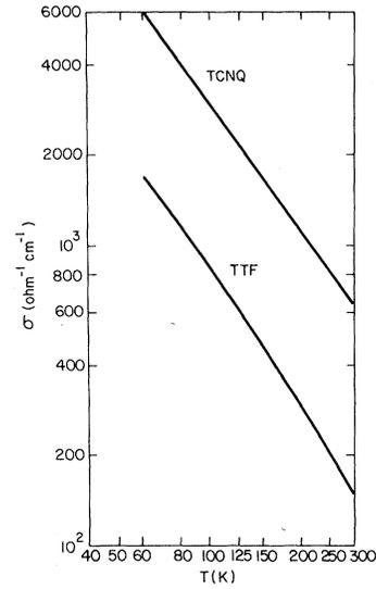
FIG. 7. Separate contributions to  $\sigma$  at constant volume of the TTF and TCNQ chains for the calculation with  $1p$  and  $2p$  processes (case II).
