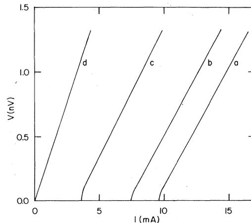
FIG. 1. Current-voltage characteristics for a junction with  $d_N = 3.8 \mu\text{m}$ . Curve a is for 4.19 K and  $H = 0$ ; b is for 4.40 K and  $H = 0$ ; c is for 4.19 K and  $H = 1$  Oe; d is for 6.55 K and  $H = 0$ .
