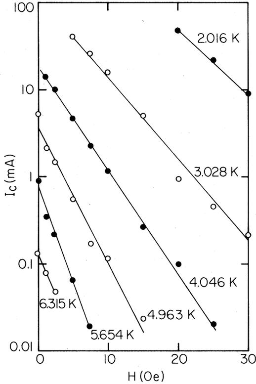
FIG. 5. Variation of  $I_c$  vs  $H$  at several temperatures for a junction of  $d_N = 34 \mu\text{m}$ .
