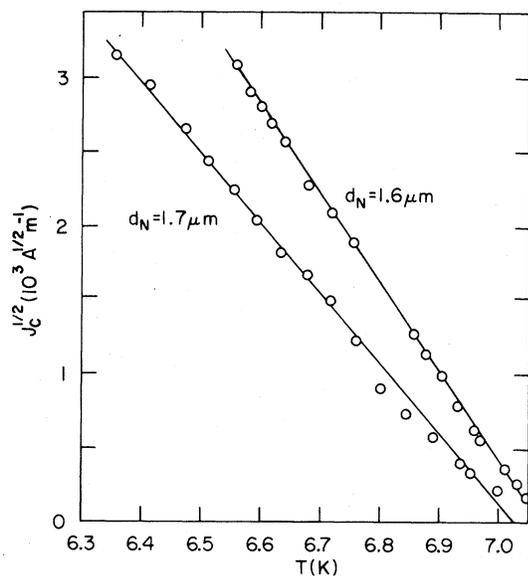
FIG. 2.  $J_c^{1/2}$  for two junctions showing the temperature dependence of  $J_c$  near  $T_{cS}$  is  $(1 - T/T_{cS})^2$ .
