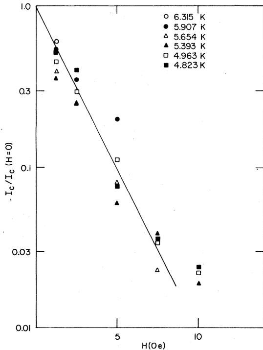
FIG. 7.  $J_c(H)/J_c(0)$  vs  $H$  at several temperatures. Deviation from the universal solid line [Eq. (4.20)] is random below 7 Oe. Deviation from linearity is in agreement with Eq. (4.19).
