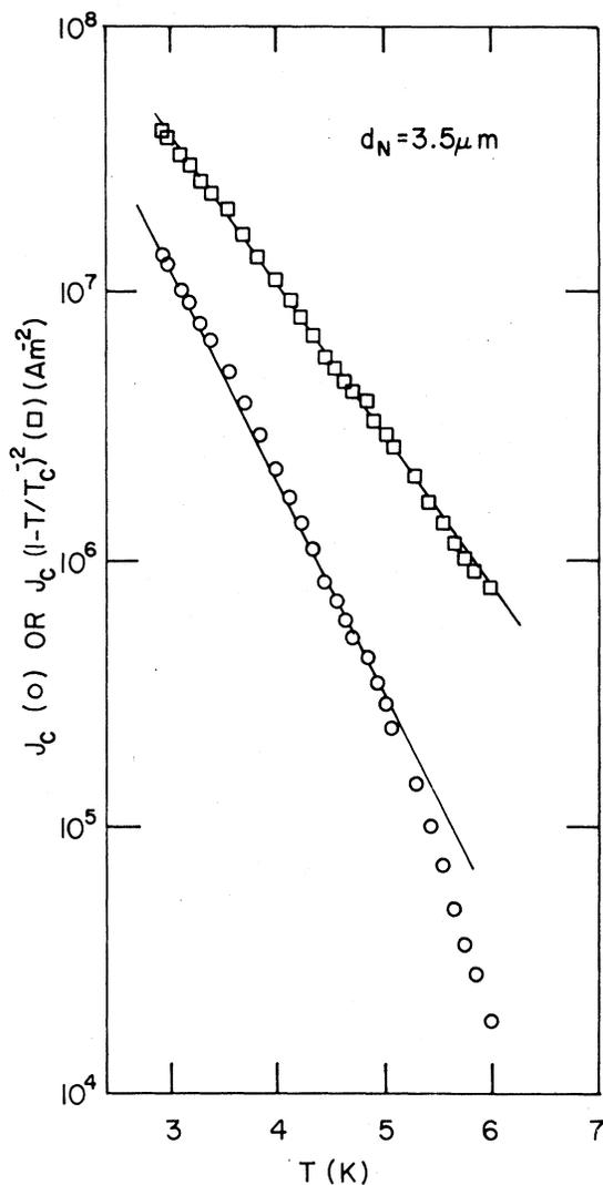
FIG. 4.  $J_c$  vs  $T$  (O) for one junction with intermediate thickness of Cd layer. Also shown is  $J_c(1 - T/T_{cS})^{-2}$  (□). Straight lines are drawn through the majority of the data points for purposes of comparison.
