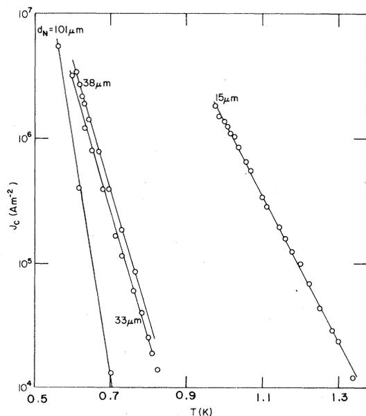
FIG. 3.  $J_c$  vs  $T$  at low temperatures for four junctions with very thick Cd layer.
