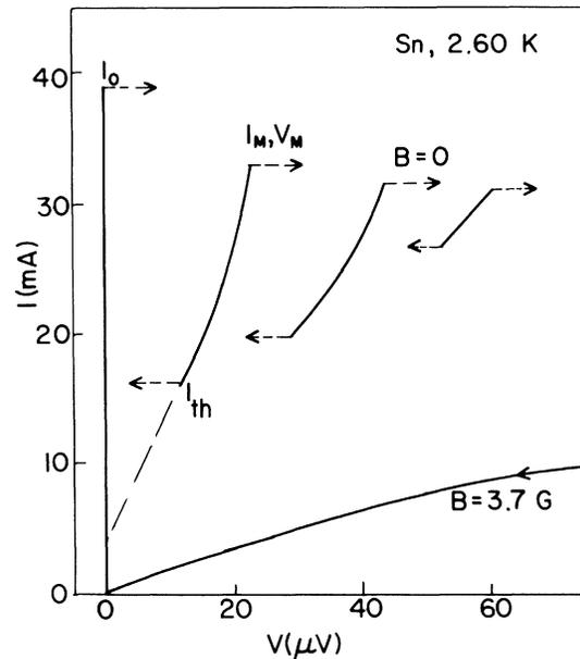
FIG. 1. The  $I$ - $V$  characteristic of a long Sn-Sn oxide-Sn junction showing three resistive branches. Junction parameters are: length  $L = 1.0$  mm, width  $W = 0.1$  mm, and  $L/\lambda_J = 31$  at 2.60 K. [ $\lambda_J$ , 0.032 mm, was calculated from  $I_0 = 4\lambda_J W j_0$  and  $\lambda_J = (\Phi_0/2\pi\mu_0 j_0 d)^{1/2}$ , where  $j_0$  is the maximum Josephson current density and  $d$  is twice the London penetration depth, about 850 Å.]
