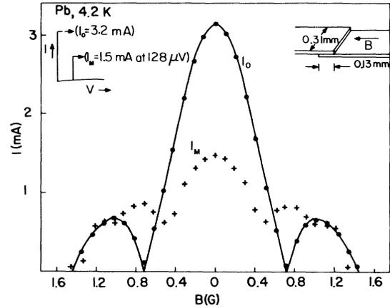
FIG. 5. Magnetic field dependences of zero-voltage current (dots) and first current singularity (crosses) of a small Pb junction. Solid line is the theoretical  $I_0$  vs  $B$ . The left inset shows the  $I$ - $V$  curve with one CS, and the right inset shows the junction geometry. At 4.2 K,  $\bar{c} = 1.92 \times 10^7$  m/s,  $j_0 = 8 \times 10^4$  A/m<sup>2</sup>, and  $\lambda_J = 0.185$  mm.
