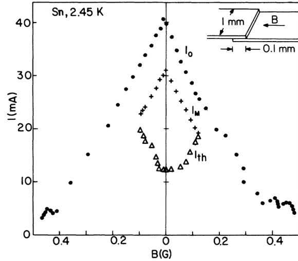
FIG. 3. The magnetic field dependences of  $I_0$ ,  $I_{\max}$ , and  $I_{th}$  as defined in Fig. 1. Inset shows the geometry of the sample and the direction of the applied magnetic field.
