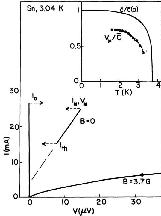
FIG. 2. The  $I$ - $V$  characteristic of the same junction as in Fig. 1 at a higher temperature, 3.04 K.  $L/\lambda_J = 24$ . Inset shows the temperature dependence (Ref. 3) of  $\bar{c}(T)/\bar{c}(0) = [1 - (T/T_c)^4]^{1/4}$  and  $v_{\max}(T)/\bar{c}(T)$ , where  $\bar{c}(0) = 1.7 \times 10^7$  m/s. The dashed line is a visual fit to the experimental data.
