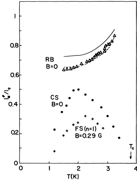
FIG. 4.  $I_{\max}^*$  vs  $T$ , where triangles are for the first RB, dots for the first CS (at the voltage of the second FS) and the crosses for the first FS. Solid and dashed lines are  $(1 - v_{\max}^2/c^2)^{1/2}$  as explained in the text.  $I_{\max}^*$  is  $I_{\max}$  minus the quasiparticle current.
