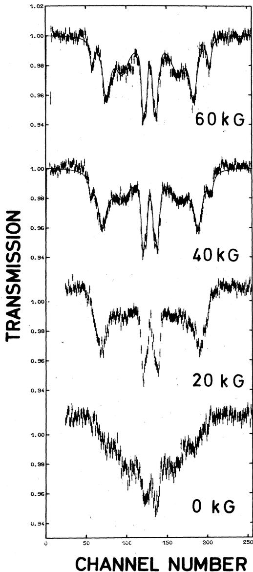
FIG. 2. Mössbauer spectra in the presence of longitudinal fields up to 80 kG at 100 K. The solid curve represents the sum of three-component spectra  $A$ ,  $B_1$ , and  $B_2$  which are theoretically simulated using the stochastic model of ionic spin relaxation and parameters described in Table I.  $\Delta V = 0.097$  mm/sec.
