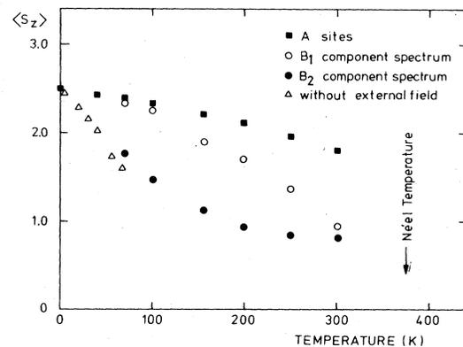
FIG. 4. Temperature dependences of  $\langle S_z \rangle$  characterizing  $A$ ,  $B_1$ , and  $B_2$  component spectra in the field of 80 kG obtained using Eq. (4) given in the text.
