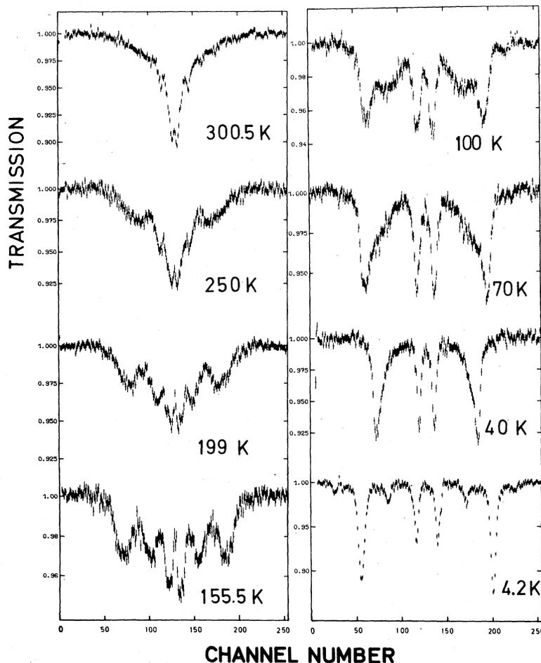
FIG. 3. Spectral shapes at temperatures in the range from 4.2 to 300 K in external field of 80 kG obtained after subtracting theoretical spectra corresponding to  $\text{Fe}^{3+}$  at  $A$  sites from the experimental spectra shown in Fig. 1.
