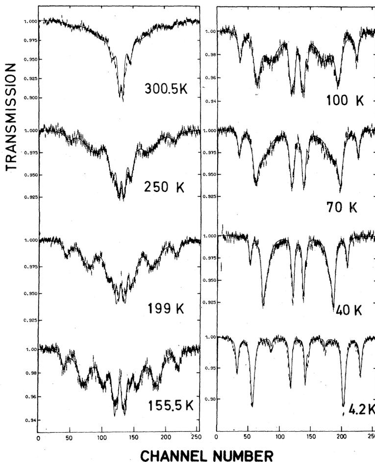
FIG. 1. Mössbauer spectra in the temperature range from 4.2 to 300 K in the presence of a longitudinal field of 80 kG. The solid curve represents the sum of three-component spectra  $A$ ,  $B_1$ , and  $B_2$  which are theoretically simulated using the stochastic model of ionic spin relaxation, described in the text. The change in velocity per channel  $\Delta V$ , in all spectra except the spectrum at 40 K is 0.097 mm/sec.
