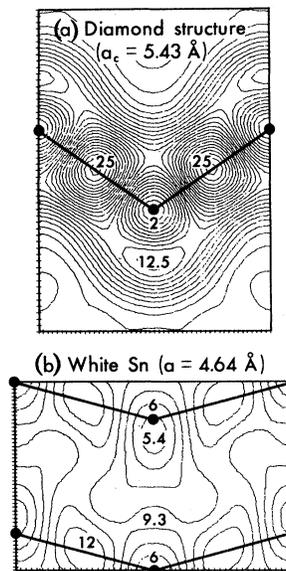
FIG. 2. The total valence charge density contours of bulk Si for (a) the diamond structure at  $\alpha_c = 5.43$  Å, and (b) the white Sn structure at  $\alpha = 4.64$  Å. Plots are in (110) plane for the diamond and in (010) plane for the white Sn structure. Heavy dots represent atomic sites, and solid lines connect nearest neighbors. Normalization corresponds to eight electrons per unit cell. Successive contours are separated by 1. The figures are plotted on the same scale for comparison.
