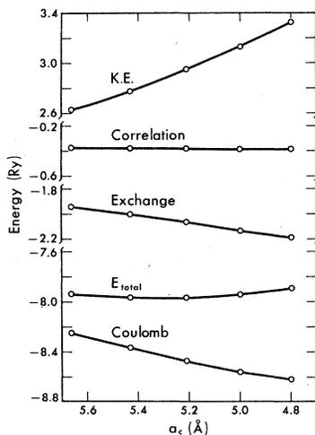
FIG. 1. Behavior of various components of the crystal energy of Si [entering Eq. (2)] as a function of the lattice constant.  $\alpha_1 Z$ ,  $\gamma_{\text{Ewald}}$ , the Hartree energy, and the ion-electron interaction energy are considered together and denoted by "Coulomb" in the figure. This plot is for the diamond structure with  $\alpha = \frac{2}{3}$ . Note how small the variation of  $E_{\text{total}}$  is compared with each component.
