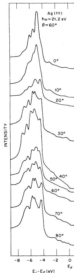
FIG. 7. Angular dependent EDC's of Ag(111) for h\nu = 21.2 eV. The incident angle of the light is kept constant at 60^\circ . All angles are measured from the surface normal and in the (\bar{1}\bar{1}2) plane.
