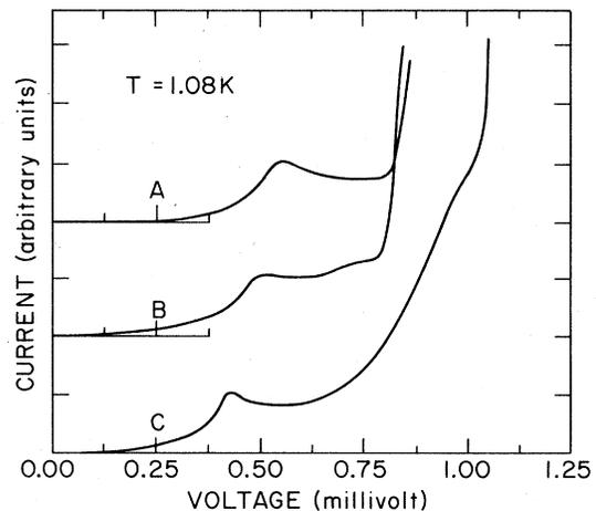
FIG. 1.  $I$ - $V$  characteristic curves, obtained at a temperature of 1.1 K. Sample *A* is a pure indium sample. Samples *B* and *C* are composed of indium with 22 atomic parts per million (ppm) of manganese.
