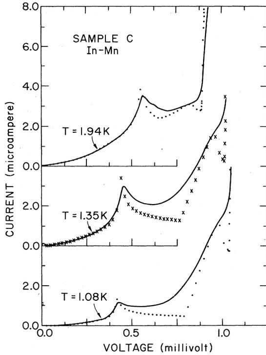
FIG. 3. Solid curves show the experimental  $I$ - $V$  curves of sample C. The points show the corresponding theoretical results according to Shiba's theory with only  $s$ -wave scattering.
