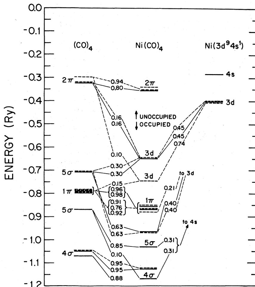
FIG. 2. Energy eigenvalues of the orbitals of  $(\text{CO})_4$ ,  $\text{Ni}(\text{CO})_4$  and  $\text{Ni}(3d^9 4s^1)$ . Labeled in terms of their main CO or Ni character. Also shown are all the squares of overlaps which are larger than 0.10. Levels of  $e$  symmetry are labeled by dashed lines, those of  $a_1$  and  $a_2$  symmetry are labeled by full lines. Parameters used in the calculation are shown in Table I.
