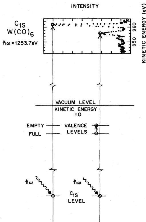
FIG. 1. Above, the  $C_{1s}$  region of the photoelectron spectra of  $W(CO)_6$  excited with  $Mg K\alpha$  radiation from Ref. 3. Below, an interpretation of the peaks in a one-electron picture.
