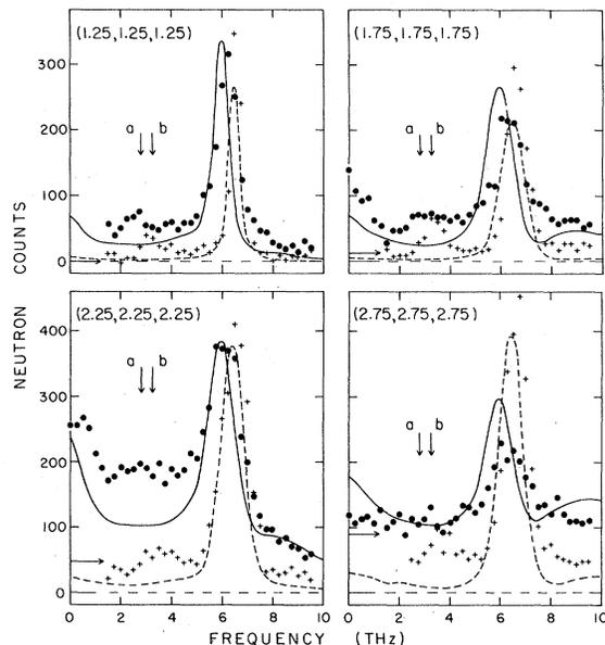
FIG. 3. The self-consistent-phonon theory  $S(\vec{Q}, \omega)$ , folded with the instrumental resolution function, at  $T = 800$  K (solid lines) and  $T = 300$  K (dashed lines) compared with the observed scattering intensity as in Fig. 1. The horizontal arrows show the part of the theoretical  $S(\vec{Q}, \omega)$  estimated to be three-phonon scattering at  $T = 800$  K.
