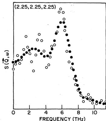
FIG. 2. Computer simulation of  $S(\vec{Q}, \omega)$  at  $\vec{Q} = (2.25, 2.25, 2.25)2\pi/a$  in Al at 800 K by Fourier transformation with an 0.5 psec damping function (solid circles). For comparison we also show the original undamped response of Ref. 20 (open circles) from the bottom left panel of Fig. 1.
