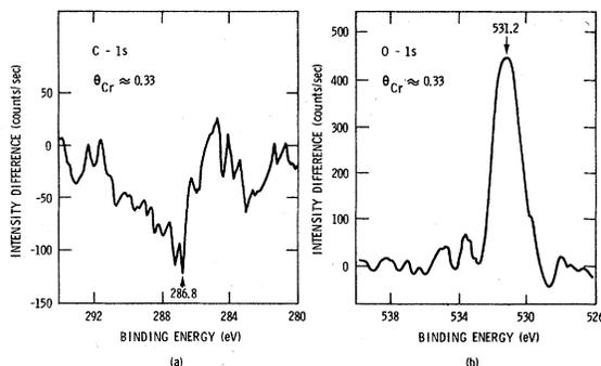
FIG. 10. (a) Difference spectrum in the carbon-1s energy region between a chromium-covered and a clean polyvinyl-alcohol surface. (b) Difference spectrum in the oxygen-1s energy region between a chromium-covered and a clean polyvinyl-alcohol surface. The chromium coverage  $\theta_{Cr}$  is 0.33 monolayer.
