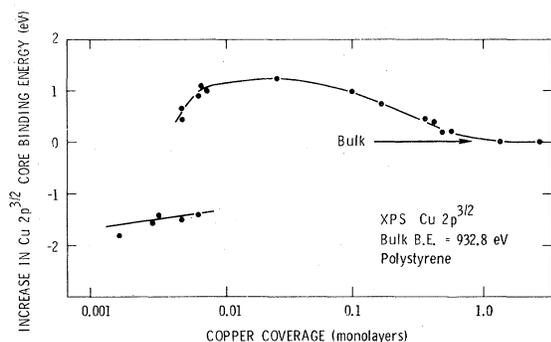
FIG. 1. Variation in the  $2p^{3/2}$  electron core binding energy as a function of metal coverage on polystyrene for deposited Cu.
