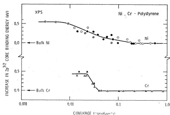
FIG. 2. Variation in the  $2p^{3/2}$  electron core binding energy as function of metal coverage on polystyrene for deposited Ni and Cr. The different-labeled points are for separate and independent metal evaporations.
