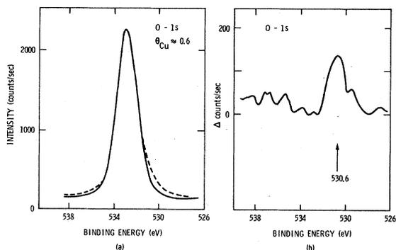
FIG. 8. (a) Oxygen-1s spectrum of a clean (solid curve) and a copper-covered (dotted curve) polyvinyl-alcohol surface. (b) Difference spectrum in the oxygen-1s energy region between a copper-covered and a clean polyvinyl-alcohol surface. The copper coverage  $\theta_{Cu}$  is 0.6 monolayer.
