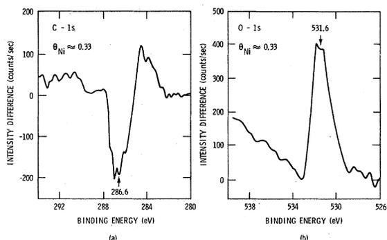
FIG. 9. (a) Difference spectrum in the carbon-1s energy region between a nickel-covered and a clean polyvinyl-alcohol surface. (b) Difference spectrum in the oxygen-1s energy region between a nickel-covered and a clean polyvinyl-alcohol surface. The nickel coverage  $\theta_{Ni}$  is 0.33 monolayer.
