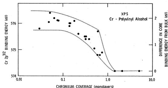
FIG. 5. Variation in the  $2p^{3/2}$  electron core binding energy as a function of metal coverage on polyvinyl alcohol for deposited Cr.
