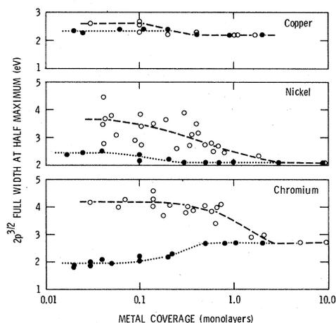
FIG. 6. Variation in the FWHM of the  $2p^{3/2}$  electron core levels as a function of metal coverage on polystyrene (full circles) and on polyvinyl alcohol (open circles) for deposited Cu, Ni, and Cr.
