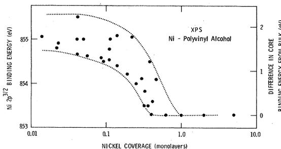
FIG. 4. Variation in the  $2p^{3/2}$  electron core binding energy as a function of metal coverage on polyvinyl alcohol for deposited Ni.
