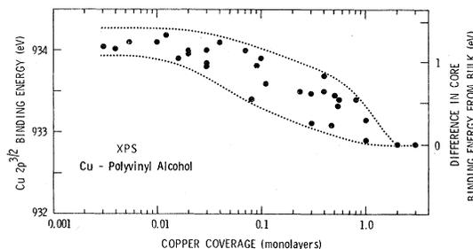
FIG. 3. Variation in the  $2p^{3/2}$  electron core binding energy as a function of metal coverage on polyvinyl alcohol for deposited Cu.
