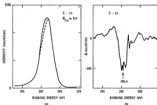
FIG. 7. (a) Carbon-1s spectrum of a clean (solid curve) and a copper-covered (dotted curve) polyvinyl-alcohol surface. (b) Difference spectrum in the carbon-1s energy region between a copper-covered and a clean polyvinyl-alcohol surface. The copper coverage  $\theta_{Cu}$  is 0.6 monolayer.
