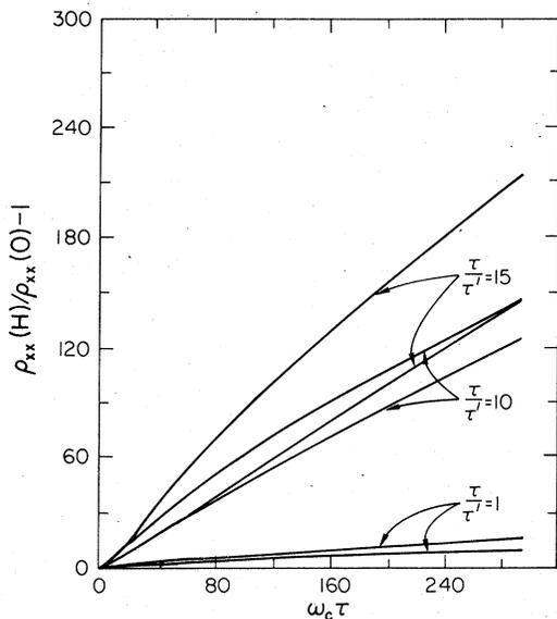
FIG. 7.  $\Delta\rho_{xx}(H) = [\rho_{xx}(H) - \rho_{xx}(0)]/\rho_{xx}(0)$  for the polycrystal with extended orbits, as described in the text. The calculations are carried out in the EMT for geometries (a) and (b), as shown in Fig. 1.  $\tau'/\tau$  is the ratio of the relaxation time for small angle scattering to that for scattering from spherical sections of the Fermi surface. For each value of  $\tau'/\tau$ , results for geometry (b) lie *above* those for (a).
