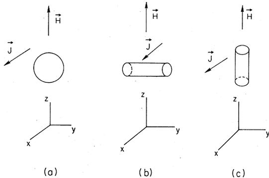
FIG. 1. Crystallite shapes in relation to direction of magnetic field and current flow for calculations described in the text. Configurations (a), (b), and (c) represent a spherical crystallite, a cylindrical one with axis perpendicular to  $\vec{H}$ , and a cylinder with axis parallel to  $\vec{H}$ , respectively.
