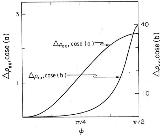
FIG. 3.  $\Delta\rho_{xx}(\omega_c\tau=200)$  for a volume fraction  $f=0.01$  of open-orbit crystallites embedded in a free-electron metal. The azimuthal angle is described in the text, and configurations (a) and (b) are exhibited in Fig. 1. The remainder of the "rotation" diagram can be obtained from the figure by means of the symmetry relations  $\Delta\rho_{xx}(\omega_c\tau, \phi) = \Delta\rho_{xx}(\omega_c\tau, \phi + \pi) = \Delta\rho_{xx}(\omega_c\tau, \pi - \phi)$ .
