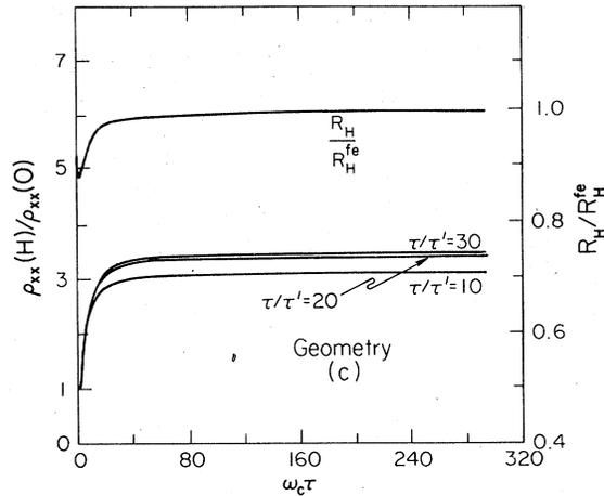
FIG. 8.  $\Delta\rho_{xx}(\omega_c\tau)$  and  $R_H/R_H^{fe}$  for the extended-orbit model of Sec. V, as calculated within the EMT for geometry (c). The strong field dependence at  $\omega_c\tau \lesssim 40$  results from the fact that the model is based on an asymptotic, high-field evaluation of the Shockley tube integral formal for the magnetoconductivity tensor.
