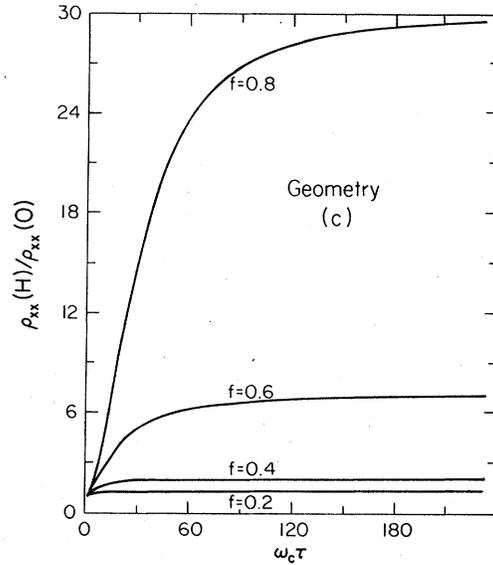
FIG. 4.  $\rho_{xx}(H)/\rho_{xx}(0)$  for a volume fraction  $f$  of open-orbit crystallites embedded in a free-electron metal, as calculated in the EMT. Configurations (a), (b), and (c) are as in Fig. 1.
