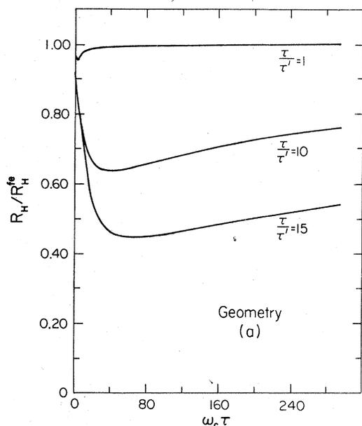
FIG. 9.  $R_H/R_H^0$  for the extended-orbit model of Sec. V for geometry (a), as calculated in the EMT. The low-field results ( $\omega_c \tau \lesssim 40$ ) are anomalous for the same reasons as in Fig. 8.
