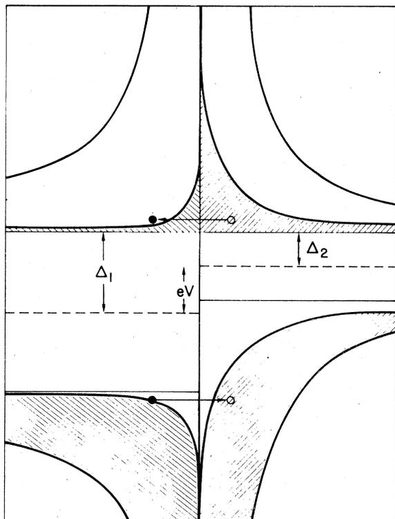
FIG. 1. Semiconductor model of tunneling between two superconducting films with  $\Delta_1 > \Delta_2$ , biased at a voltage  $V = (\Delta_1 - \Delta_2)/e$ . The upper arrow indicates "electron" tunneling, and the lower "hole" tunneling.
