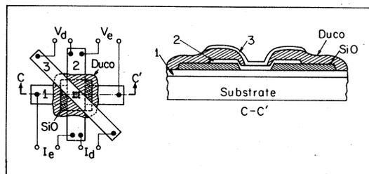
FIG. 2. (Left) plan view of sample configuration; (right) section  $cc'$  of sample (film thicknesses greatly exaggerated). Width of films 1 and 3 is 3 mm.
