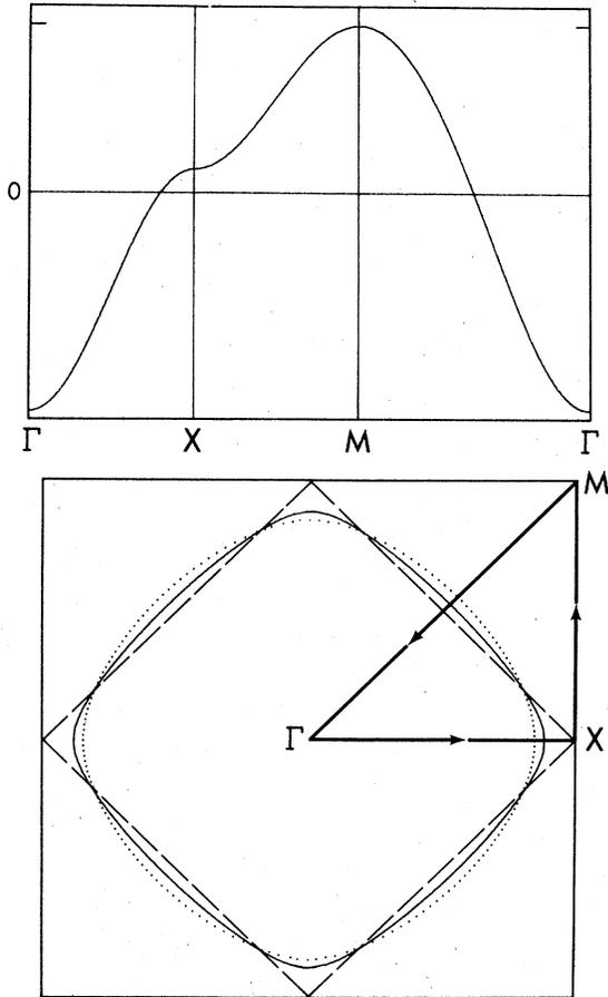
FIG. 1. (a) Band structure of the two-dimensional square lattice for  $t_1/t_0 = 0.25$ . (b) The Fermi surface for the two-dimensional square lattice and a half-filled band. The dashed line is for  $t_1/t_0 = 0$ , the full line for  $t_1/t_0 = 0.125$ , and the dotted line for  $t_1/t_0 = 0.25$ .
