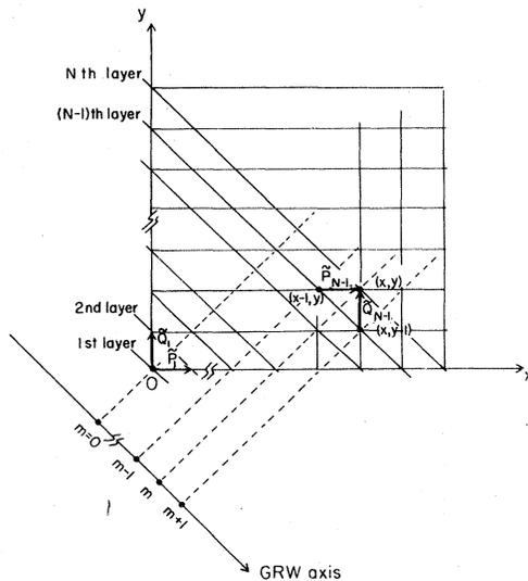
FIG. 2. Relation between a special walk process specified by Eqs. (2.7), (2.9), and (2.10) and a generalized-random-walk process given by Eqs. (3.2), (3.3), and (3.4).
