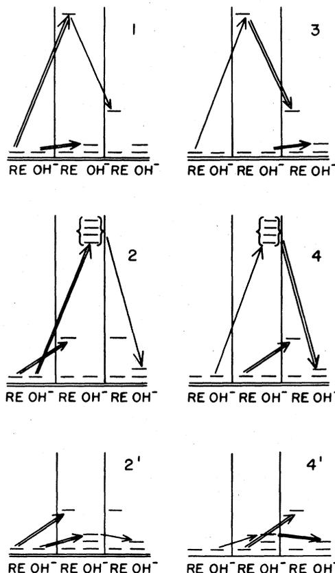
FIG. 2. Schematic representation of initial, intermediate, and final states for a cooperative absorption process. Double arrows correspond to electrostatic interactions, single arrows to radiative matrix elements.
