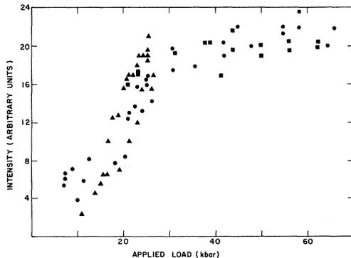
FIG. 3. Intensity of the nuclear-resonance free-induction-decay amplitude versus applied load at 6.9 MHz and  $T = 4.2$  °K. The triangles refer to an initial loading to 26 kbar, the circles to a loading of a new sample to 65 kbar, and the squares to a first loading two days later.
