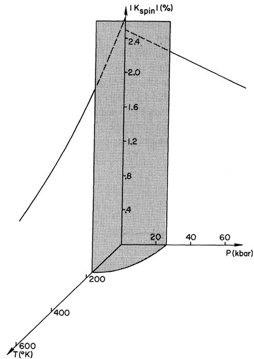
FIG. 4.  $d$ -spin components of  $^{51}\text{V}$  NMR frequency shifts as a function of pressure at  $T = 4.2^\circ\text{K}$  and as a function of temperature at  $P = 1 \text{ atm}$ . The solid lines are linear and Curie-Weiss fits, respectively, of the data. The broken lines are continuations of the fits in the anti-ferromagnetic region where no resonances were observed.
