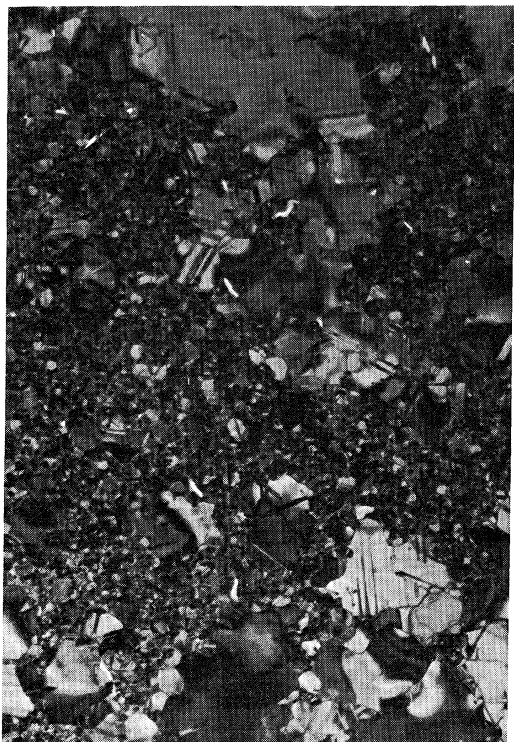
FIG. 2. Transmission electron micrograph of a non-annealed Au film ( d=232 \text{ \AA} ).
