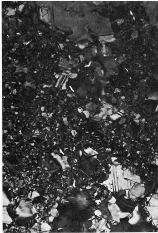
FIG. 2. Transmission electron micrograph of a non-annealed Au film ( d = 232 \text{ \AA} ).
