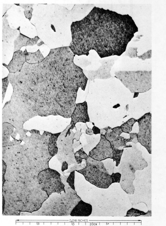
FIG. 1. Transverse section of quenched Ni 3 Fe specimen etched with ammonium persulfate ( \times 200 original magnification). Difference in brightness of grains is due to orientation differences, including twinning.
