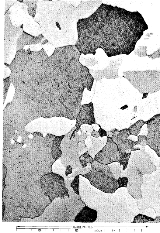
FIG. 1. Transverse section of quenched \text{Ni}_3\text{Fe} specimen etched with ammonium persulfate ( \times 200 original magnification). Difference in brightness of grains is due to orientation differences, including twinning.
