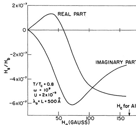
FIG. 3. Real and imaginary parts of  $H_s/H_b$  as a function of  $H_0$  with  $N(0) = 10^{34}$  (cm<sup>3</sup>erg)<sup>-1</sup> for case (a) (rf field on one side).  $H_c$  for Al with these parameters is 165 G.
