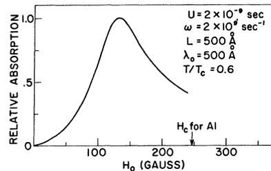
FIG. 1. Shape of an absorption curve for case (b), the case for which the rf field is equal on both sides of the film. It is essentially Lorentzian except for the extra factor of  $H_{0\text{av}}$  which causes asymmetry.  $H_c$  for Al with these parameters is 247 G.
