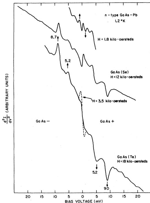
FIG. 6. Tunneling spectra from Pb junctions on *n*-type GaAs showing the normal Pb phonons at  $-8.7$ ,  $-5.2$  and at  $+9.0$ ,  $+5.2$  mV. The upper curve for GaAs(Se) and the dotted curve for GaAs(Te) show incomplete quenching of the lead gap at lower magnetic fields.
