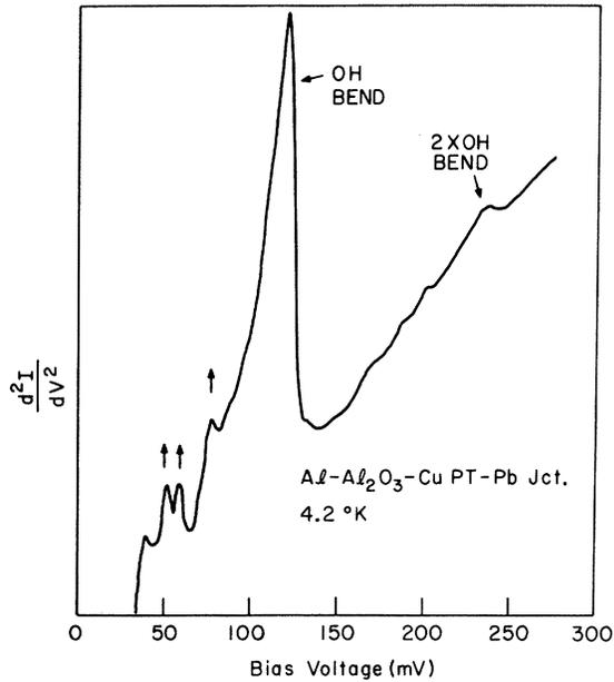
FIG. 17. Tunneling spectra of Al-Al<sub>2</sub>O<sub>3</sub>-Pb junction doped with phthalocyanine after Jaklevic and Lambe (Ref. 36).
