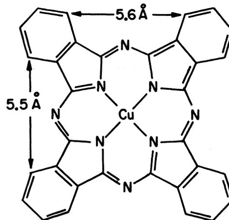
FIG. 16. Structure of copper-phthalocyanine ( $\text{C}_8\text{H}_4\text{N}_2$ )<sub>4</sub>Cu.
