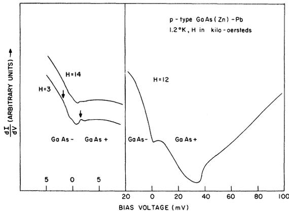
FIG. 10. Conductance or  $dI/dV$  of a Pb junction in the normal state on  $p$ -type GaAs (Zn)-Pb at  $1.2^\circ\text{K}$ . The curves on the left show the effect of magnetic field in reducing the structure left over from the quenched Pb gap.
