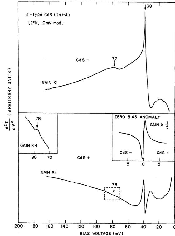
FIG. 12. Tunneling spectra from Au junction on  $n$ -type CdS(In) at  $1.2^\circ\text{K}$ . Structure occurs at the LO phonon energy ( $\pm 38$  mV) and at twice the LO phonon energy in both forward and reverse bias.
