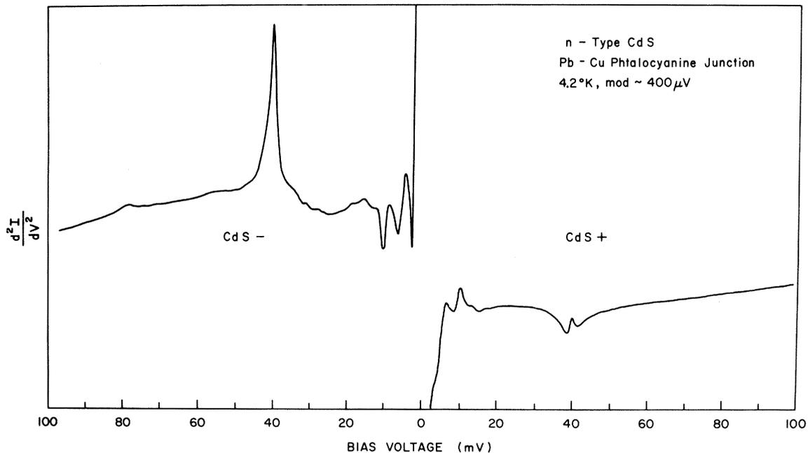
FIG. 19. Tunneling spectra from Pb junction on *n*-type CdS doped with copper phthalocyanine at 4.2 °K.
