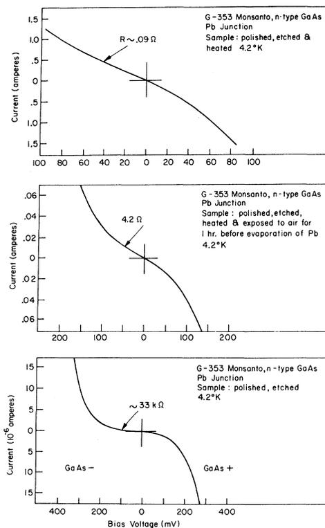
FIG. 1. Effect of surface preparation of GaAs on the current-voltage characteristics of the Pb-GaAs junctions at 4.2 °K. The carrier concentration of the *n*-type GaAs(Se) is  $5.5 \times 10^{18}$  cm<sup>-3</sup>. The lowest junction impedances are obtained on samples heated in vacuum before evaporation of the metal electrodes.
