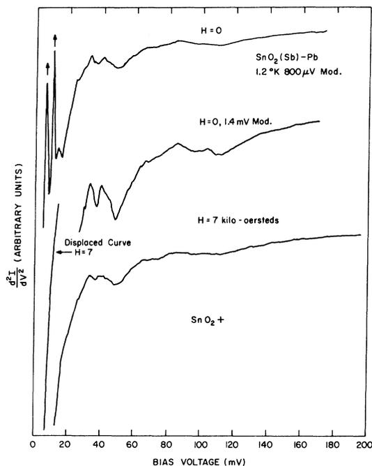
FIG. 15. Tunneling spectra of the  $\text{SnO}_2$ -Pb junction at  $1.2^\circ\text{K}$  in reverse bias.
