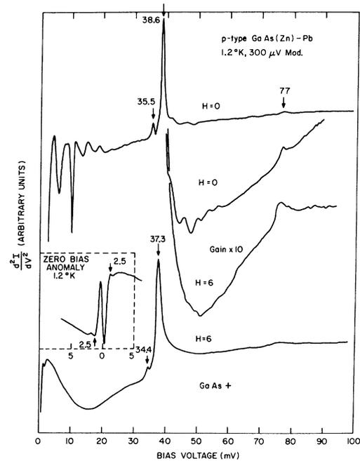
FIG. 9. Tunneling spectra from Pb junction on  $p$ -type GaAs(Zn) at forward bias at 1.2 °K. Structure at high-energy side of GaAs phonons ( $H=0$ ) is due to reflection of superconducting density-of-states structure of Pb between 6 and 20 mV. The peak at 77 mV corresponds to twice the energy of the GaAs 1.0 phonon. The insert shows the structure due to a resistance maximum and incomplete quenching of the lead gap ( $H=6$  kOe) at zero bias.
