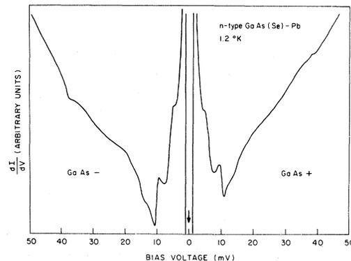
FIG. 7. Conductance or  $dI/dV$  of a typical Pb junction on *n*-type GaAs at  $1.2$  K. The arrow at zero bias points to the large decrease in conductance due to the superconducting lead gap. The structure at  $\pm 38$  mV is due to LO phonon of GaAs.
