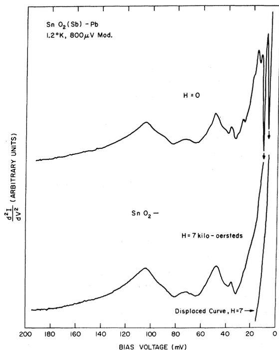
FIG. 14. Tunneling spectra of an  $n$ -type  $\text{SnO}_2(\text{Sb})$ -Pb junction at  $1.2^\circ\text{K}$  at forward bias. In the lower curve the superconducting lead density-of-states phonons at 6 and 10 mV has been quenched by the magnetic field.
