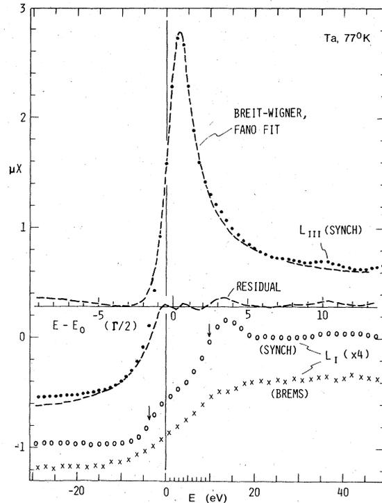
FIG. 3. Ta  $L_{III}$  edge ( $\bullet$  synchrotron data) as fitted with a Breit-Wigner-Fano-type line shape and a residual part in dashed curves. The latter is compared with the  $L_I$  edges ( $\times 4$ ):  $\times$  from the bremsstrahlung source, with the inflection point lined up at  $E=0$ ; and  $\circ$  from the synchrotron source, lined up with the previous data but with the two inflection points (designated by arrows) occurring below and above zero.
