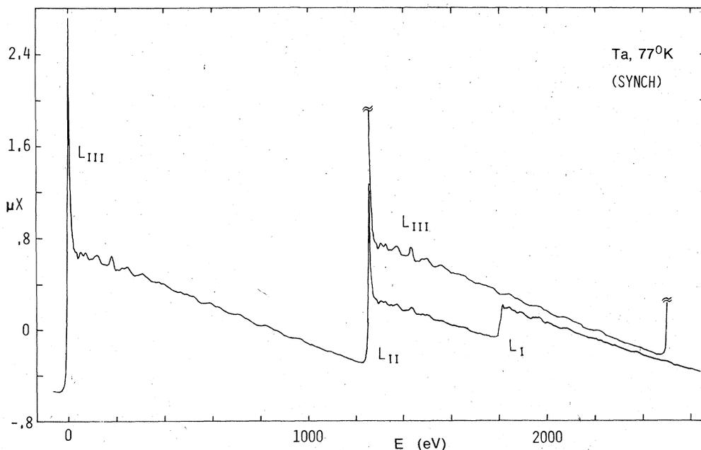
FIG. 1. X-ray absorption spectrum at the  $L$  edges of tantalum measured from a synchrotron source. The sharp spikes at the  $L_{\text{II}}$  and  $L_{\text{III}}$  edges are called white lines for a historical reason. The x-ray energy scale is plotted relative to the  $L_{\text{III}}$  edge which occurs at 9881.1 eV. For comparison, the  $L_{\text{III}}$  absorption fine structure is replotted above the  $L_{\text{II}}$  and  $L_{\text{I}}$  edges.
