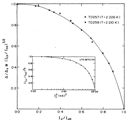
FIG. 6. Injector current dependence of the normalized energy gap exhibiting a second-order phase transition for several proximity-effect bridges.
