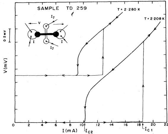
FIG. 1.  $I$ - $V$  characteristics of a typical proximity-effect bridge (TD 259) at two different temperatures. The inset shows the sample geometry: dark areas—tin; light areas—silver;  $\times$  indicate solder contacts of electrical leads.
