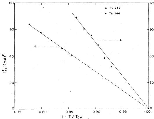
FIG. 4. Variation of the square of the second critical current with bath temperature for two typical proximity-effect bridges.
