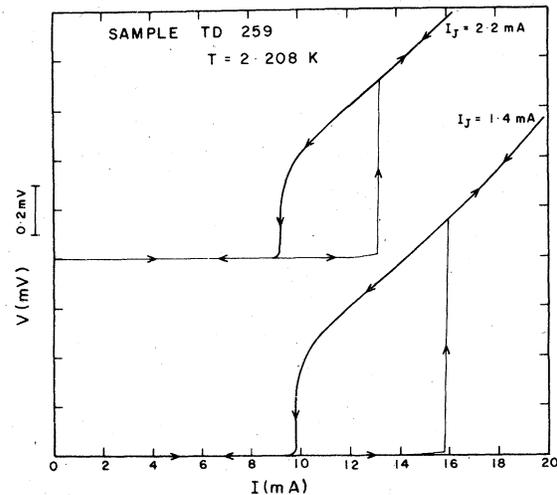
FIG. 3.  $I$ - $V$  characteristics of a typical proximity-effect bridge (TD 259) for two different injector currents at  $T = 2.208$  K.
