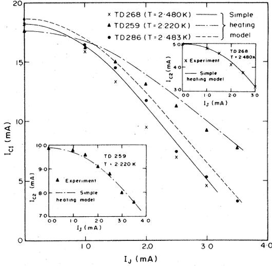
FIG. 5. Injector current dependence of the critical currents for a few proximity-effect bridges.
