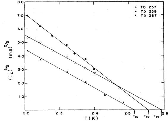
FIG. 2. Critical-current dependence on bath temperature for a few proximity-effect bridges.
