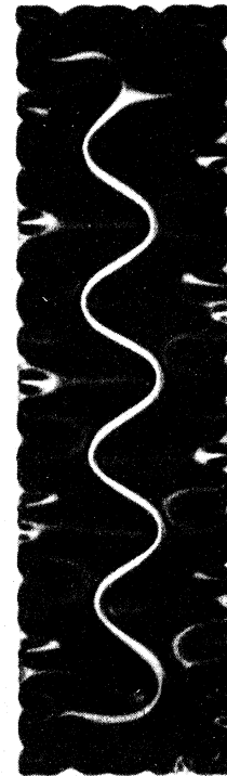
FIG. 2. Photograph of a membrane measuring 1.0 \times 0.25 mm, showing the sinusoidal pattern produced by microscope light interference in the slightly wrinkled \text{SiO}_2 film.
