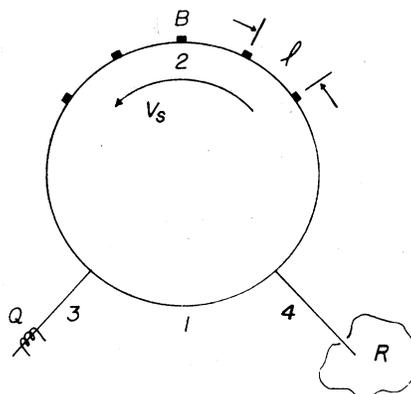
FIG. 1. Schematic of the persistent current film flow path. The Pyrex annular ring has a diameter of approximately 10 cm. The reservoir R consists of 8 g of  $\text{Al}_2\text{O}_3$  powder (0.05  $\mu\text{m}$ ) and provides a large surface area to stabilize the film thickness.
