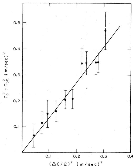
FIG. 2. Typical example of the observed  $C_3^2 - C_{30}^2$  plotted against the observed  $(\frac{1}{2} \Delta C)^2$ . The solid line is a least-squares fit to the data in this particular case (slope:  $1.36 \pm 0.05$ ). Here we have  $T = 1.27$  K and  $d = 9.4$ .
