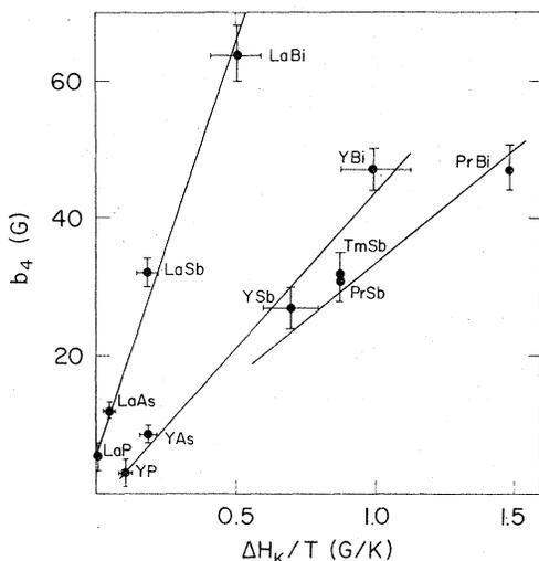
FIG. 5. Plot of  $b_4$  of Gd in the Van Vleck pnictides and in the analogous nonmagnetic pnictides versus the Korringa relaxation rates as measured for the same hosts.
