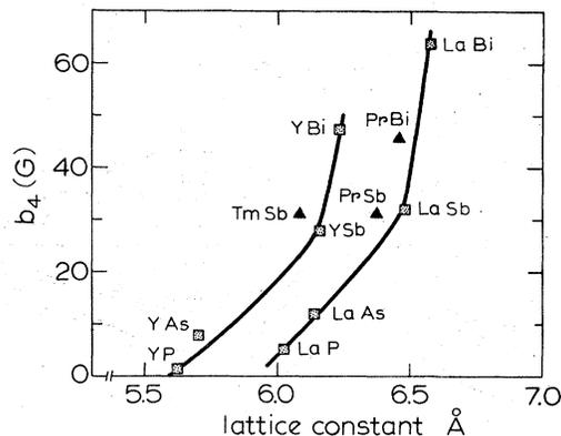
FIG. 4. Plot of the values of  $b_4$  of Gd in various pnictides vs the host lattice constant. The values of  $b_4$  for the nonmagnetic pnictides were taken from Refs. 1 and 2. The solid lines are guide to the eye.
