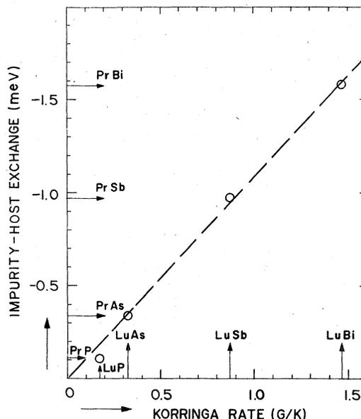
FIG. 6. Correlation between the Gd-Pr exchange interaction,  $J_{\text{Gd-Pr}}$  measured in the Van Vleck pnictides and the Gd Korringa thermal broadening,  $\Delta H_K/T$ , as measured in analogue nonmagnetic LuX ( $X = \text{P, As, Sb, Bi}$ ) pnictides.
