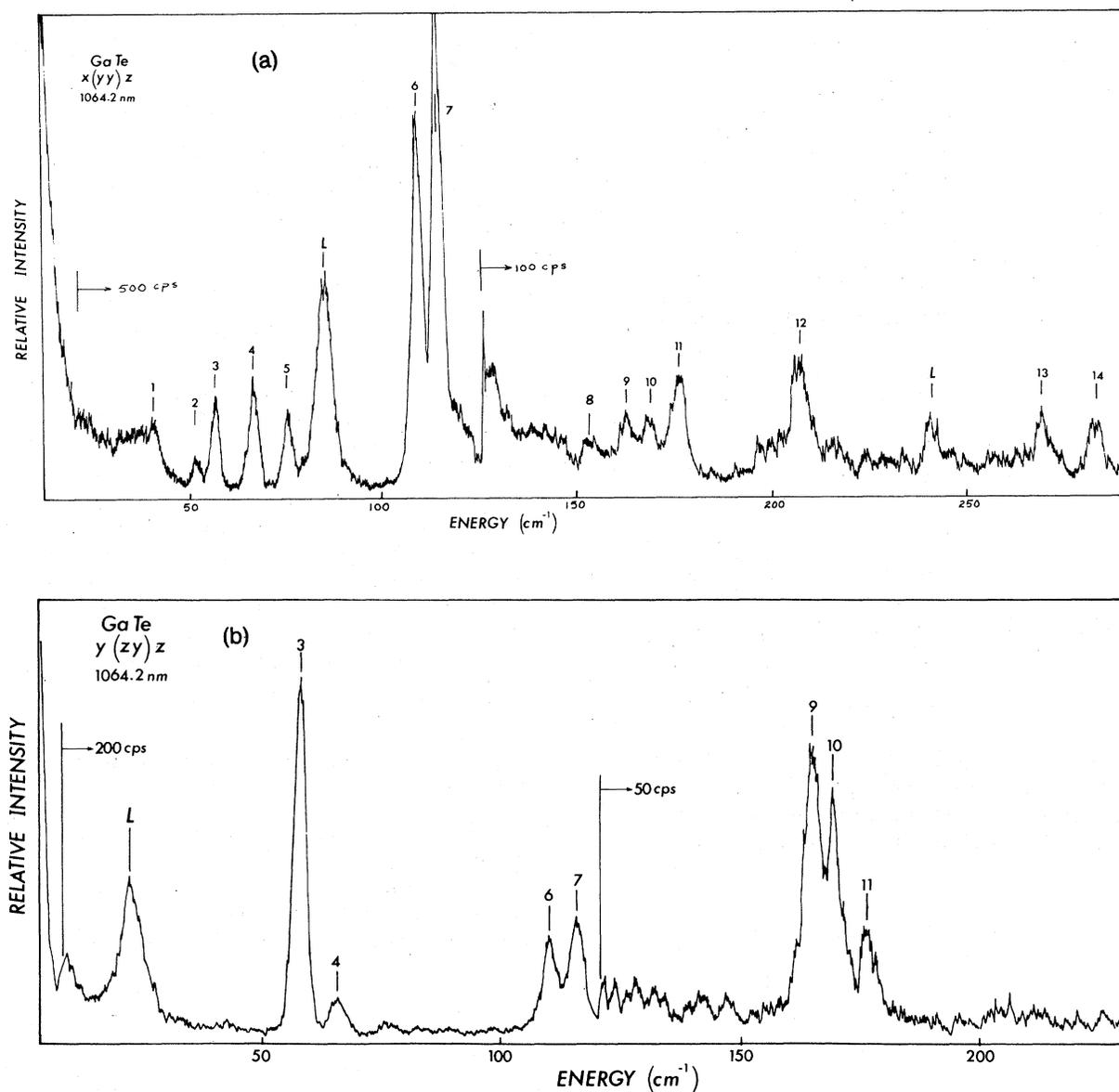
FIG. 2. Raman spectra of GaTe obtained at 300 K with the 1064.2-nm line of a YAIG: Nd<sup>3+</sup> laser and 800-mW incident intensity.
