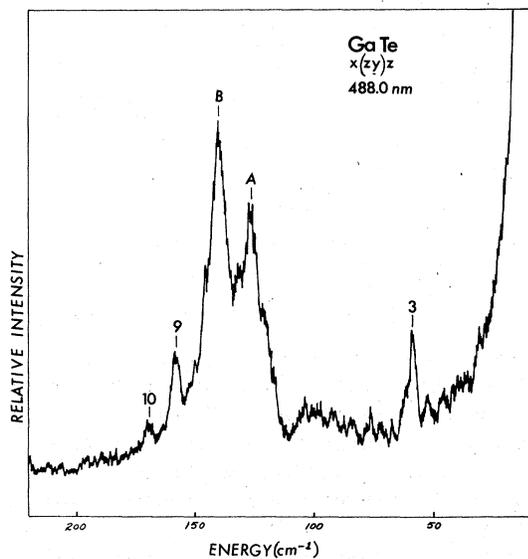
FIG. 4. Raman spectrum of GaTe obtained at 300 K with the 488.0-nm line of an argon-ion laser and 500-mW incident intensity.
