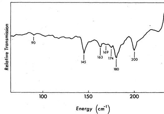
FIG. 5. Infrared absorption spectrum of GaTe obtained with the sample at 4 K and with the incident light traveling perpendicular to the plane of the layers.
