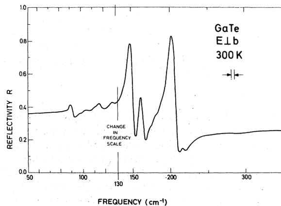
FIG. 6. Infrared reflection spectrum of GaTe obtained with the sample at 300 K and with  $E$  parallel to the crystal  $b$  axis.
