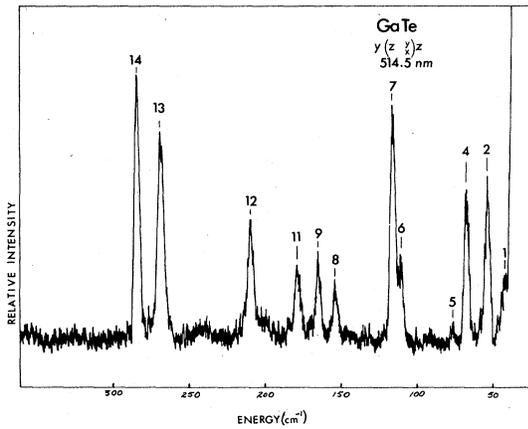
FIG. 3. Raman spectrum of GaTe obtained at 80 K with the 514.5-nm line of an argon-ion laser and 100-mW incident intensity.
