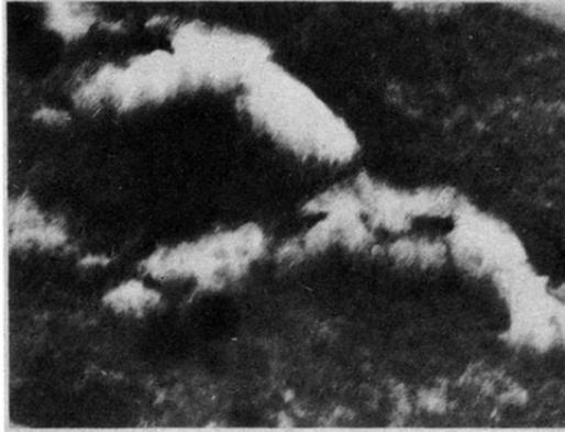
FIG. 1. Electron-microscope spectrum of sample B. The crystals appearing at the lower left of the photograph represent microcrystals of MgO of about 70 Å in size mixed in the sample for calibration purposes.
