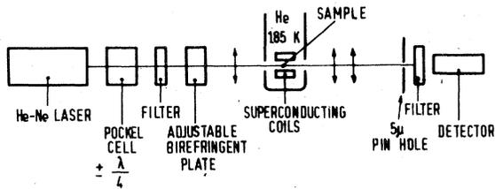
FIG. 1. Block diagram of the experimental apparatus of MCD absorption.
