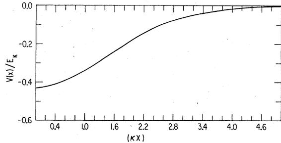
FIG. 6. Interaction potential  $V(x)$  vs  $x$  between a kink and an antikink. For small  $x$ ,  $V(x) \approx (-\frac{3}{2} + \frac{5}{96}\kappa^2 x^2)E_K$ . Whereas for large distances  $V(x) = -6E_K \exp(-\sqrt{2}\kappa x)$ .
