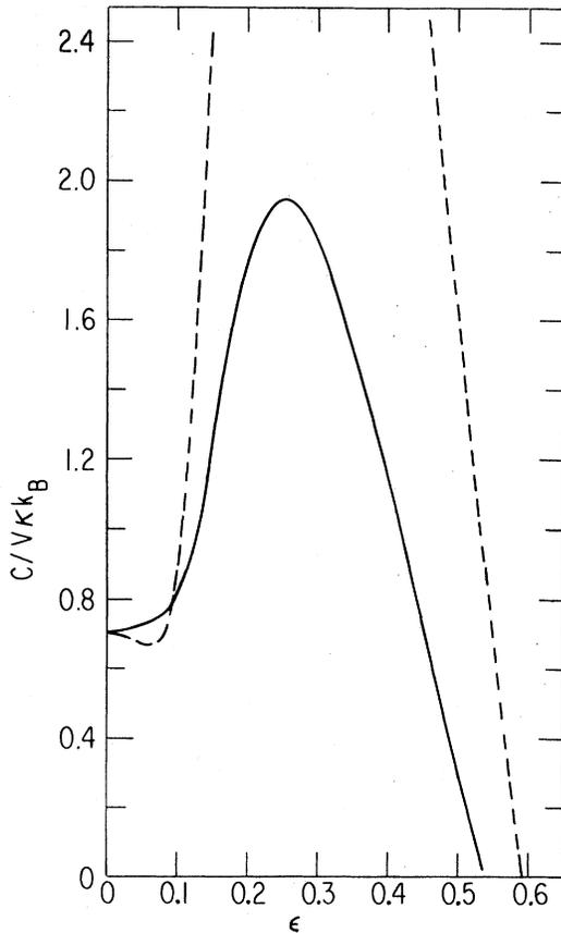
FIG. 10. Specific heat of the kink-phonon system vs  $\epsilon$  for  $\lambda=0$  (straight line) and  $\lambda=1$  (dashed line).
