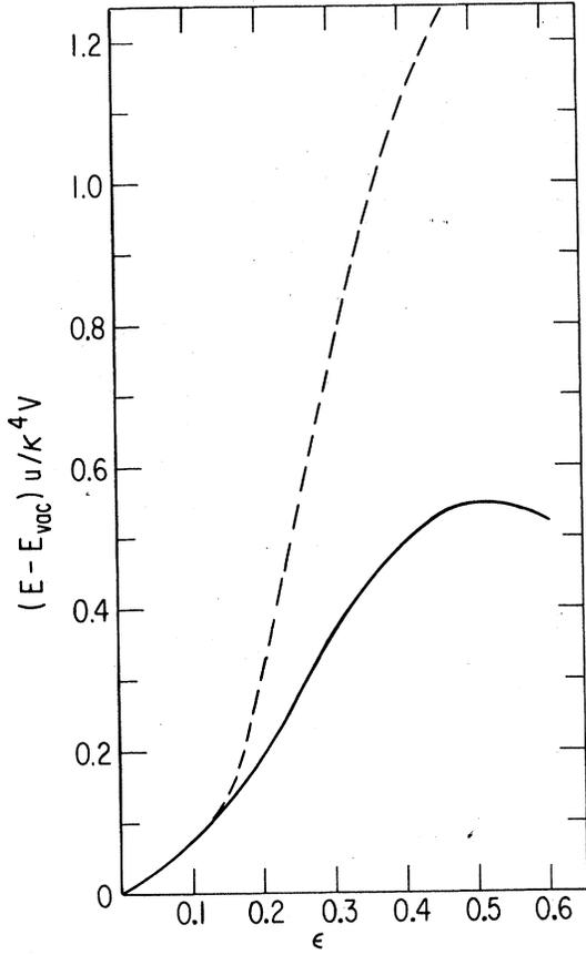
FIG. 9. Energy of the kink-phonon system vs  $\epsilon$  for  $\lambda=0$  (solid line) and  $\lambda=1$  (dashed line).
