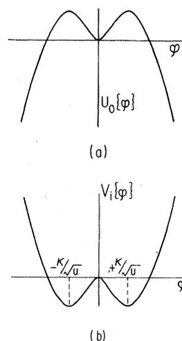
FIG. 2. (a) Symmetric potential with minimum at  $\varphi=0$  and two humps symmetrically located at  $\varphi_c^0 = \pm 1/(2\bar{g})$ . (b) Symmetric double-well potential with minima located at  $\varphi_c^0 = \pm \kappa/\sqrt{u}$ .
