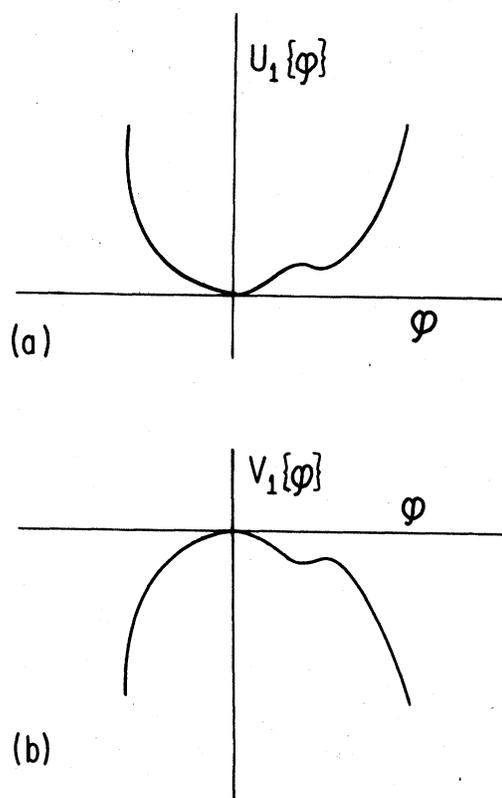
FIG. 1. (a) Potential  $U_1(\varphi)$  vs  $\varphi$  with an absolute minima at  $\varphi=0$ . (b) Potential  $V_1(\varphi) = -U(\varphi)$  vs  $\varphi$ .
