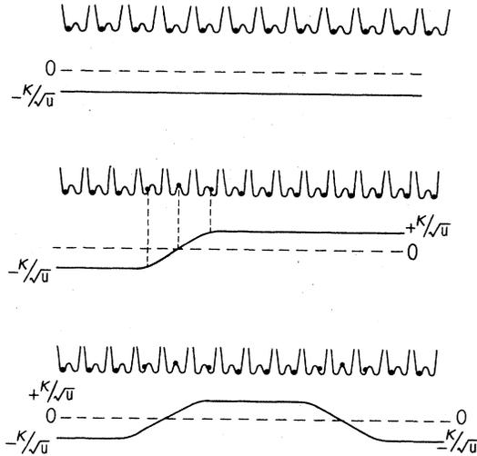
FIG. 4. (a) Classical vacuum, (b) one-kink, and (c) kink-antikink field configurations.
