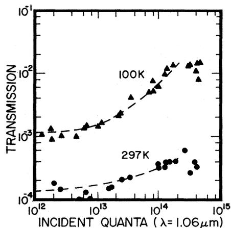
FIG. 1. Transmission of a  $5.2\text{-}\mu\text{m}$ -thick germanium sample at  $1.06 \mu\text{m}$  as a function of incident quanta at  $1.06 \mu\text{m}$  for sample temperatures of 100 and 297 K. The dashed lines are theoretical curves from Elci *et al.* (Ref. 7). The data are from Smirl *et al.* (Ref. 5).
