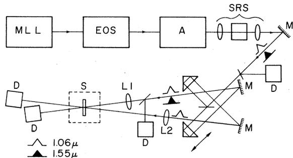
FIG. 3. Block diagram of the experimental configuration for excite and probe measurements at 1.06 and 1.55  $\mu\text{m}$ , where MLL denotes the mode-locked laser, EOS the electro-optical switch, A the laser amplifier, SRS the stimulated-Raman-scattering cell, M a mirror, D a detector, L1 and L2 lens, and S the sample.
