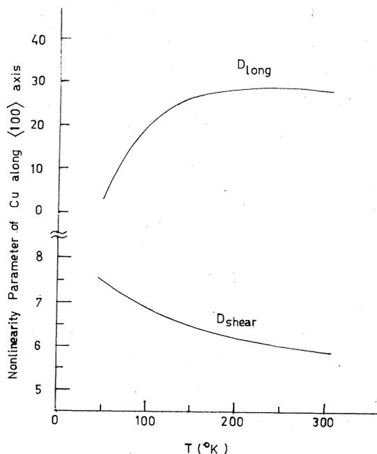
FIG. 1. Temperature variation of  $D_{\text{long}}$  and  $D_{\text{shear}}$  in copper for wave propagation along the  $\langle 100 \rangle$  axis.
