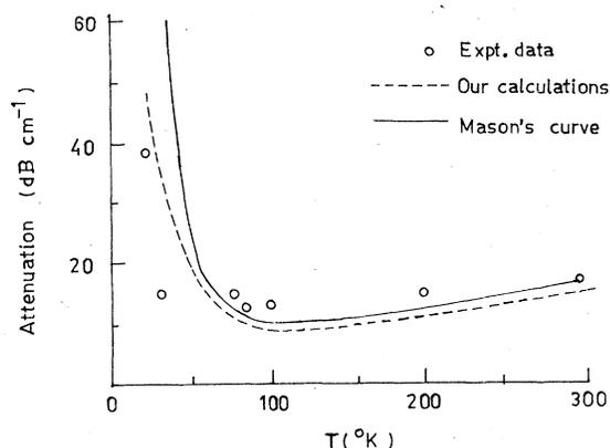
FIG. 2. Ultrasonic attenuation in copper for longitudinal wave propagation along the  $\langle 100 \rangle$  axis at 150 MHz.
