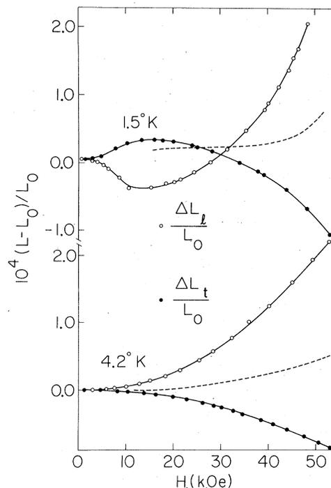
FIG. 2. Longitudinal magnetostriction (change of length parallel to field) (open circles) and transverse magnetostriction (closed circles) in the LTP (1.5 °K) and above the LTP (4.2 °K). Dotted lines: estimates of volume magnetostriction using Eq. (3a).  $L_0$  is sample length at 4.2 °K and  $H = 0$  in this and subsequent figures.
