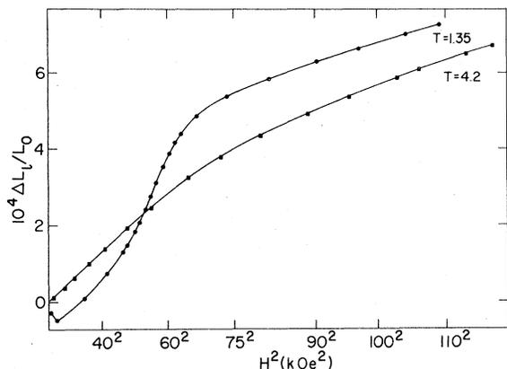
FIG. 3. Longitudinal magnetostriction versus square of magnetic field at 1.35 and 4.2 °K.
