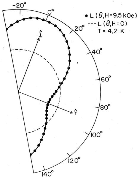
FIG. 5. Polar plot of magnetostriction (solid points) in arbitrary units versus angle of length measurement relative to applied field. The  $\hat{l}$  (longitudinal) and  $\hat{r}$  directions are indicated. The solid line is a fit to the empirical form  $A + B \cos^2 \gamma$ . The dotted line is the length in zero field.
