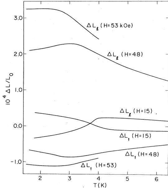
FIG. 6. Longitudinal ( $\Delta L_L$ ) and transverse ( $\Delta L_T$ ) magnetostriction versus temperature for different field values.
