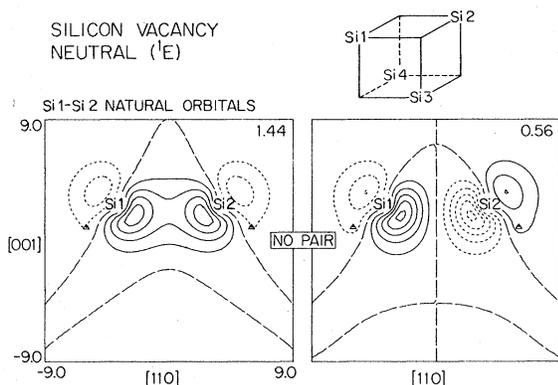
FIG. 3. The natural orbitals of one bond pair of the  ${}^1E$  state of neutral vacancy (silicon).
