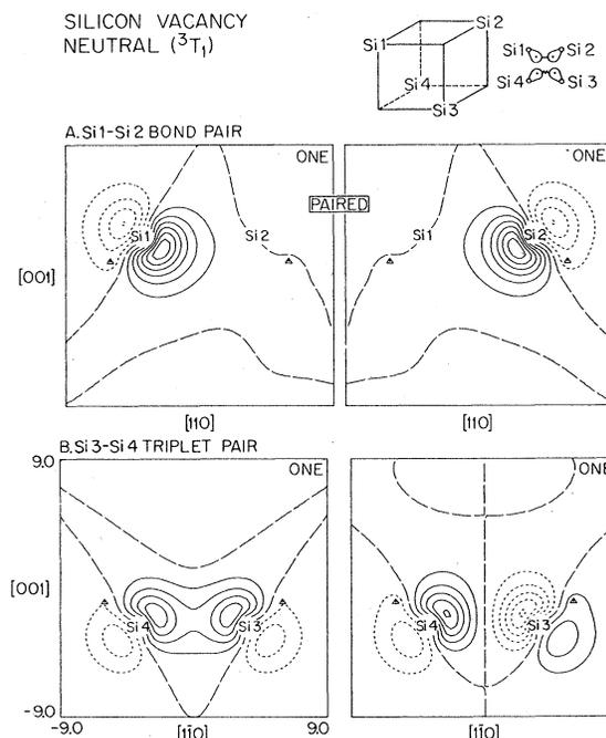
FIG. 4. The GVB orbitals of the  ${}^3T_1$  state of the neutral vacancy (silicon).
