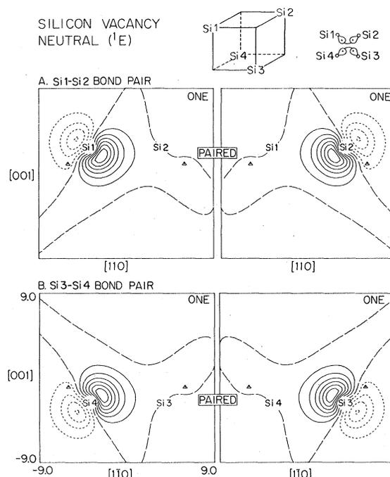
FIG. 2. Amplitudes of the GVB orbitals for the <sup>1</sup>E state of the neutral vacancy (silicon). The long dashes indicate nodal surfaces. The spacing of the contour lines is 0.03 a.u. with the dashed lines being negative. This spacing is used for all of the silicon orbitals. The centers are labeled according to Table I and Fig. 1. These conventions are used for all other plots.
