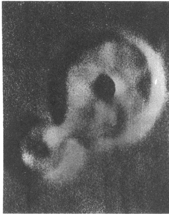
FIG. 2. Surface of a film selectively etched in NaOH as shown by the SEM (scanning electron microscope). Holes 2\ \mu\text{m} in diameter were observed where Al columns penetrated the films, and collapsed edges where the NaOH selectively etched out the Al layers.
