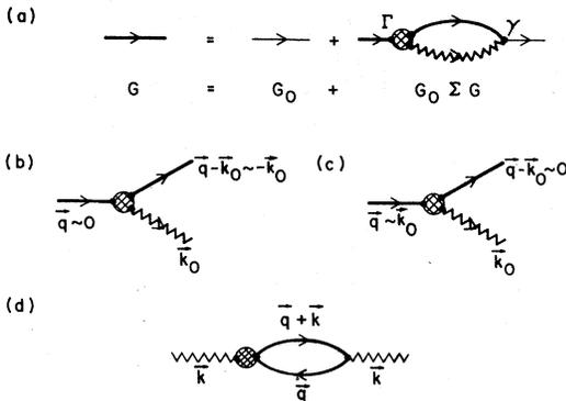
FIG. 1. (a) Dyson's equation; (b) and (c) vertices for  $q \sim 0$  and  $q \sim k_0$  quasiparticles, respectively; and (d) usual diagram for calculation of hybridization effects. Wavy and straight lines represent <sup>4</sup>He and <sup>3</sup>He propagators. Renormalized (unrenormalized) propagators are in bold (light).
