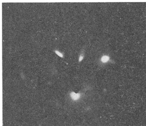
FIG. 2. Low-energy-electron-diffraction patterns of the clean \text{SrTiO}_3 (111) surface after Ar-ion bombardment at 600^\circ\text{C} and subsequent annealing at 600^\circ\text{C} . (a) E_p = 25 eV. (b) E_p = 34 eV.
