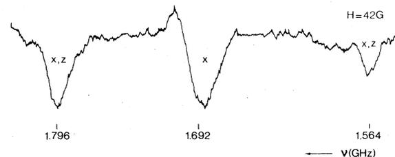
FIG. 6. ODMR spectrum of  $F$  center in CaO in the presence of a small magnetic field along  $y$  ( $H_y=42$  G). The optical polarization of the resonance lines is as indicated.
