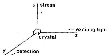
FIG. 1. Directions of the pumping light and the detected emitted light, respectively, in our axis convention.
