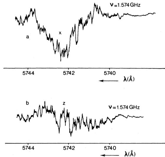
FIG. 5. Zero-phonon line in PMDR showing only  $x$  polarization [(a)  $x$  polarization; (b)  $z$  polarization], when  $H_z=38$  G,  $\nu=1.574$  GHz, and  $\vec{H}_1 \parallel \vec{x}$ .
