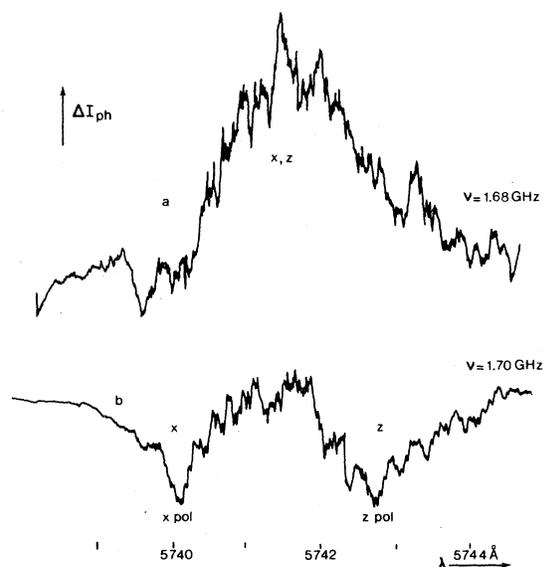
FIG. 3. (a) Zero-field PMDR spectrum showing only the zero-phonon line taken with  $\nu = 1.68 \text{ GHz}$ , the microwave  $H_1$  field being polarized (mainly) along the  $x$  axis;  $T = 1.5 \text{ K}$ . (b) Zero-field PMDR zero-phonon lines taken with  $\vec{H}_1 \parallel \vec{x}$ ,  $\nu = 1.70 \text{ GHz}$ ,  $T = 1.5 \text{ K}$ .
