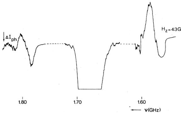
FIG. 7. ODMR spectrum of  $F$  center in CaO in the presence of a small magnetic field along  $z$  ( $H_z = 43$  G). The resonance lines at  $\nu = 1.58$  GHz and  $\nu = 1.80$  GHz partly reflect a light decrease.
