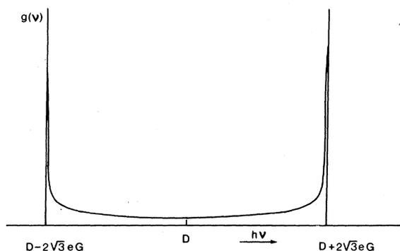
FIG. 9. Variation of the spectral density  $g(\nu)$  with the resonance frequency  $\nu$  of the  $\eta_y \rightarrow \eta_z$  ODMR transition under conditions of (i) equal probability for each  $\phi$  in the interval  $0 \leq \phi \leq 2\pi$  and (ii) a constant strain magnitude  $e$ .
