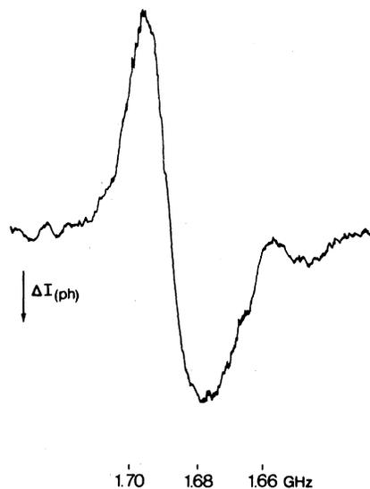
FIG. 2. Zero-field ODMR spectrum of the CaO:  $F$  center excited to its  ${}^3T_{1u}$  state. Detection wavelength  $\lambda = 5742 \text{ \AA}$ ;  $T = 1.5 \text{ K}$ .
