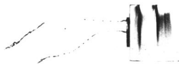
FIG. 2. Three kinds of darkening observed in an annealed crystal produced by synchronized application of pulses of electric field, light of 300–650-nm wavelength, and stationary ultrasound wave.
