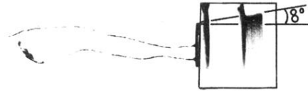
FIG. 6. Darkening in an annealed crystal produced by synchronized application of pulses of an electric field, light of 300–650-nm wavelength, and ultrasound waves.
