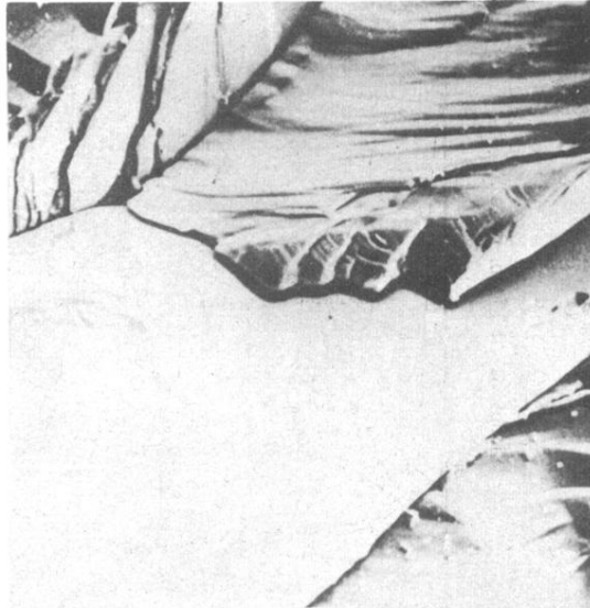
FIG. 14. Scanning electron micrograph of surfaces of crushed powder particle, showing cracks between regions of different morphology. Width of picture, 240 \mu\text{m} .
