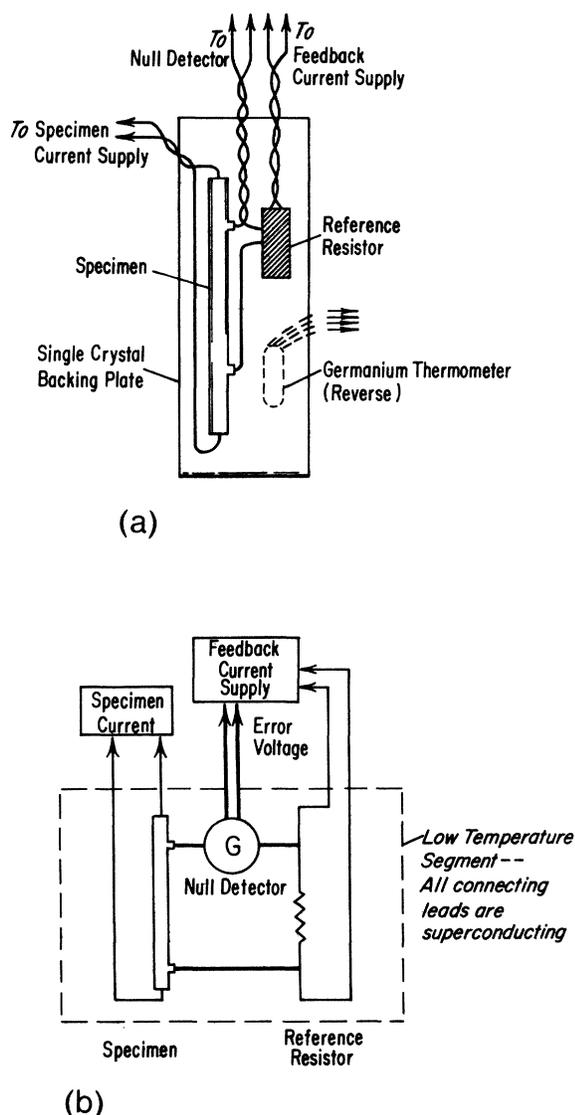
FIG. 1. (a) Detail of the specimen holder. (b) Schematic diagram of the measurement system.
