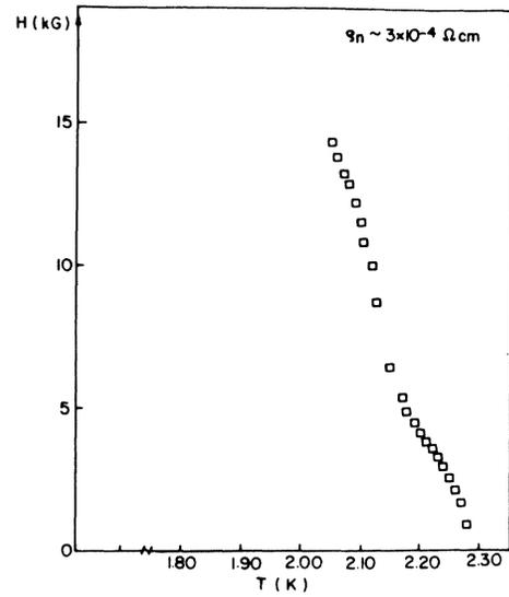
FIG. 2. Upturn in the parallel critical field observed in a granular aluminium film (after Ref. 9). The normal-state resistivity is  $\rho_n$ .
