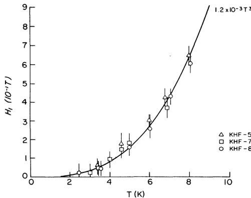
FIG. 4.  $H_1$ , the field at which  $\omega_c \tau_{th} = 1$  as a function of the temperature. The impurity contribution to  $\tau_{th}$  has been subtracted from  $H_1$ .
