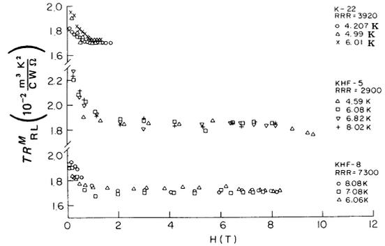
FIG. 1. Measured Righi-Leduc coefficient of potassium times the temperature as a function of the applied magnetic field; only the higher temperatures are displayed. The specimens shown are representative of the range of purity studied.
