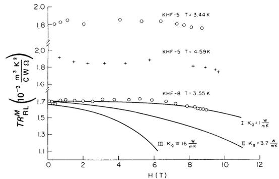
FIG. 2. Measured Righi-Leduc coefficient of potassium times the temperature as a function of the applied magnetic field, for several low temperatures. These data illustrate the field dependence of  $TR_{RL}^M$  at high fields. The curves are discussed in the text.
