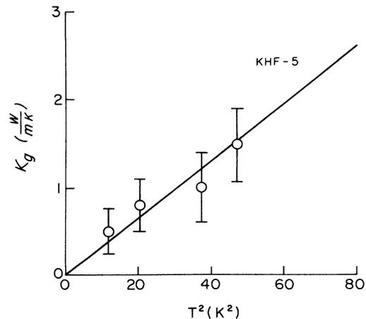
FIG. 5. Lattice thermal conductivity of the potassium as a function of the square of the temperature for specimen KHF-5. The errors are determined by the fit to the Righi-Leduc data.
