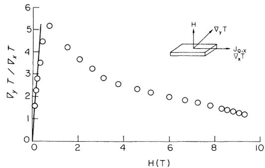
FIG. 3. Ratio of the thermal gradient perpendicular to the heat current to the thermal gradient parallel to the heat current (see inset) as a function of the applied magnetic field. The line drawn at low fields is discussed in the text.
