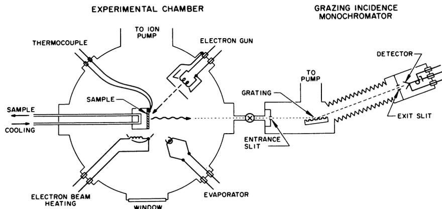
FIG. 1. Experimental apparatus for emission measurements.
