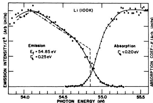
FIG. 6. Emission and absorption edge spectra taken with the NBS spectrometer reduced to be proportional to the density of states. See text for details.
