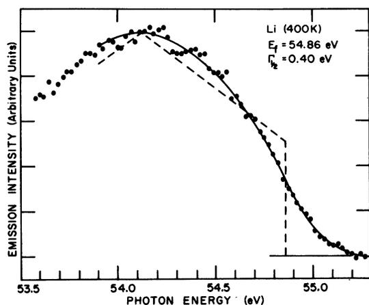
FIG. 4. X-ray emission edge of Li at 400 K. Dashed line is same unbroadened edge function shown in Fig. 3, but moved up in energy by 0.05 eV.
