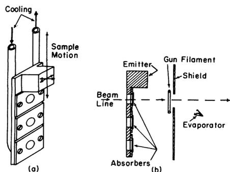
FIG. 2. (a) Sample mount for combined emission and absorption measurements. (b) Experimental arrangement of sample, evaporator, and electron gun for the combined measurements.
