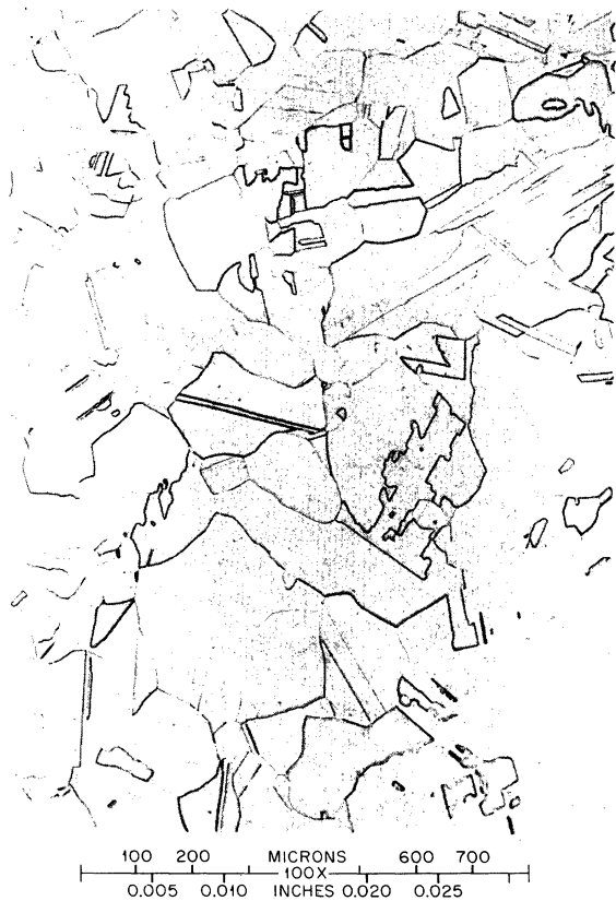
FIG. 1. Photomicrograph at 100 \times of nickel-bar stock from which specimen was made, showing microstructure typical of nickel and some nickel alloys after annealing, polishing, and etching.
