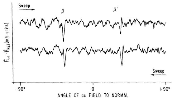
FIG. 5. Transmitted field projected upon a constant reference as a function of the orientation of the dc magnetic field to the sample surface under orientation and masking conditions of Fig. 4(b). The peaks correspond to that labeled  $\beta$  and  $\beta'$  in Fig. 1, and as can be seen are basically symmetric in amplitude. The dc magnetic field was 18 kG, temperature 1.4 K, and sample thickness 0.055 cm.
