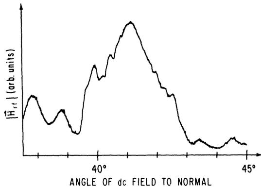
FIG. 2. Magnitude of the transmitted microwave field in the vicinity of the  $\beta$  peak of Fig. 1. The dc magnetic field was 18 kG and the temperature 1.4 K.
