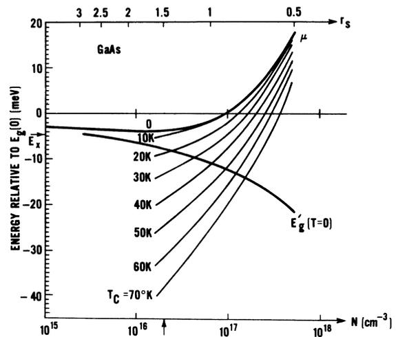
FIG. 3. Reduced band gap  $E'_g$  and carrier chemical potential  $\mu$  for  $T=0^\circ\text{K}$  as a function of carrier density. The influence of carrier temperature on chemical potential is also illustrated. The method of calculation is described in detail in the text.
