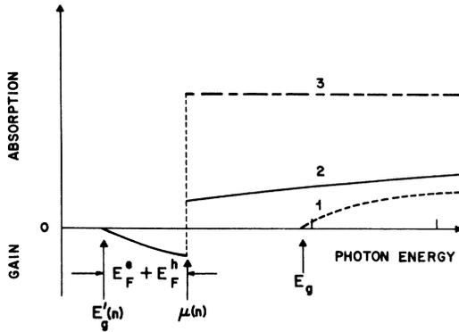
FIG. 2. Illustrative schematic of absorption coefficient at  $T=0^\circ\text{K}$  for various conditions as discussed in the text.
